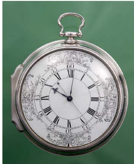
Figure 2.1 Harrison's fourth and final version of the chronometer, courtesy of the National Maritime Museum
