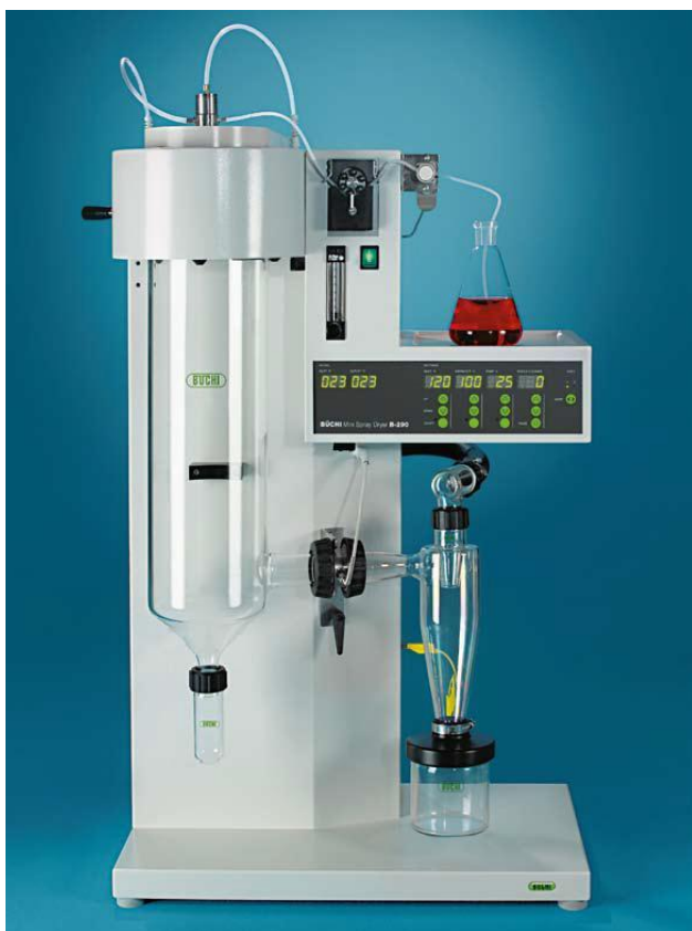
Figure 3.1. Laboratory scale bench top Spray dryer Buchi B-290 (commercial Boucher Masontechnology).
