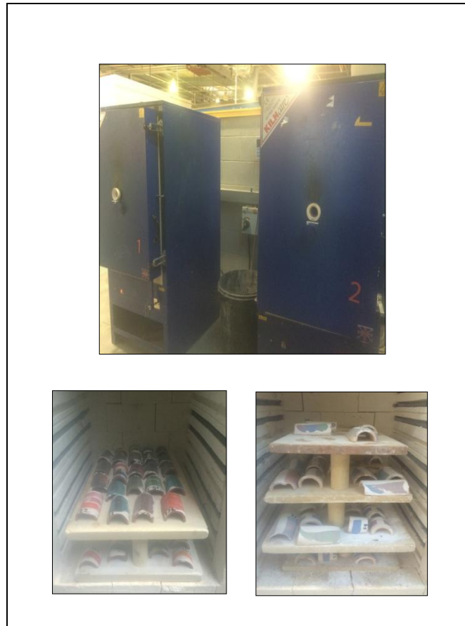
Figure 28 UOS Kiln firing with test samples for Machado palette.
