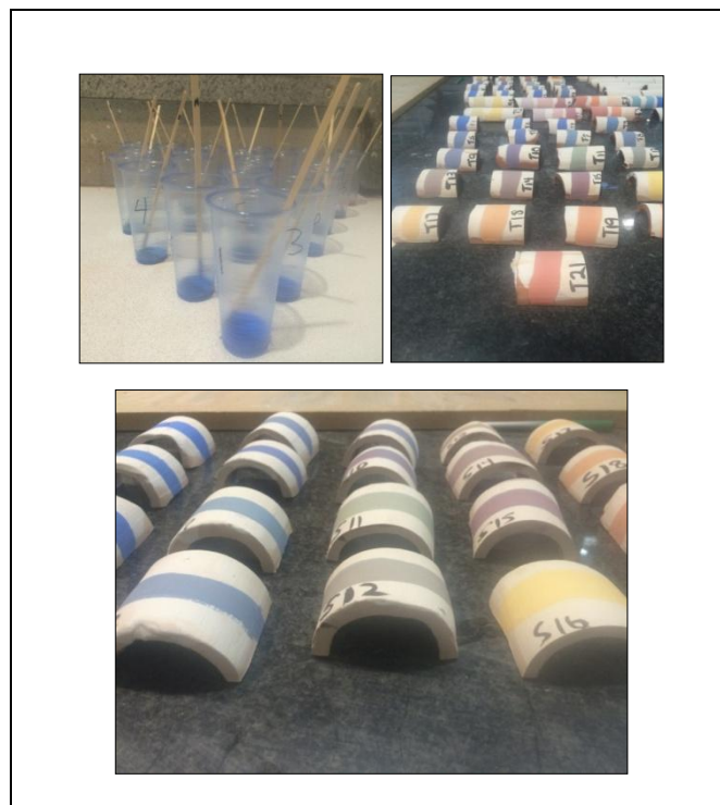
Figure 21 Triaxial combination trial
