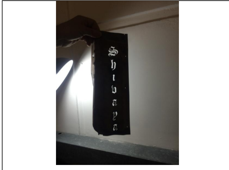
Figure 116 Snyder Tin roof jet cut sample back lit
