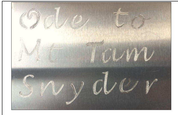
Figure 118 Snyder sample with 12V handheld engraver on zinc plate
