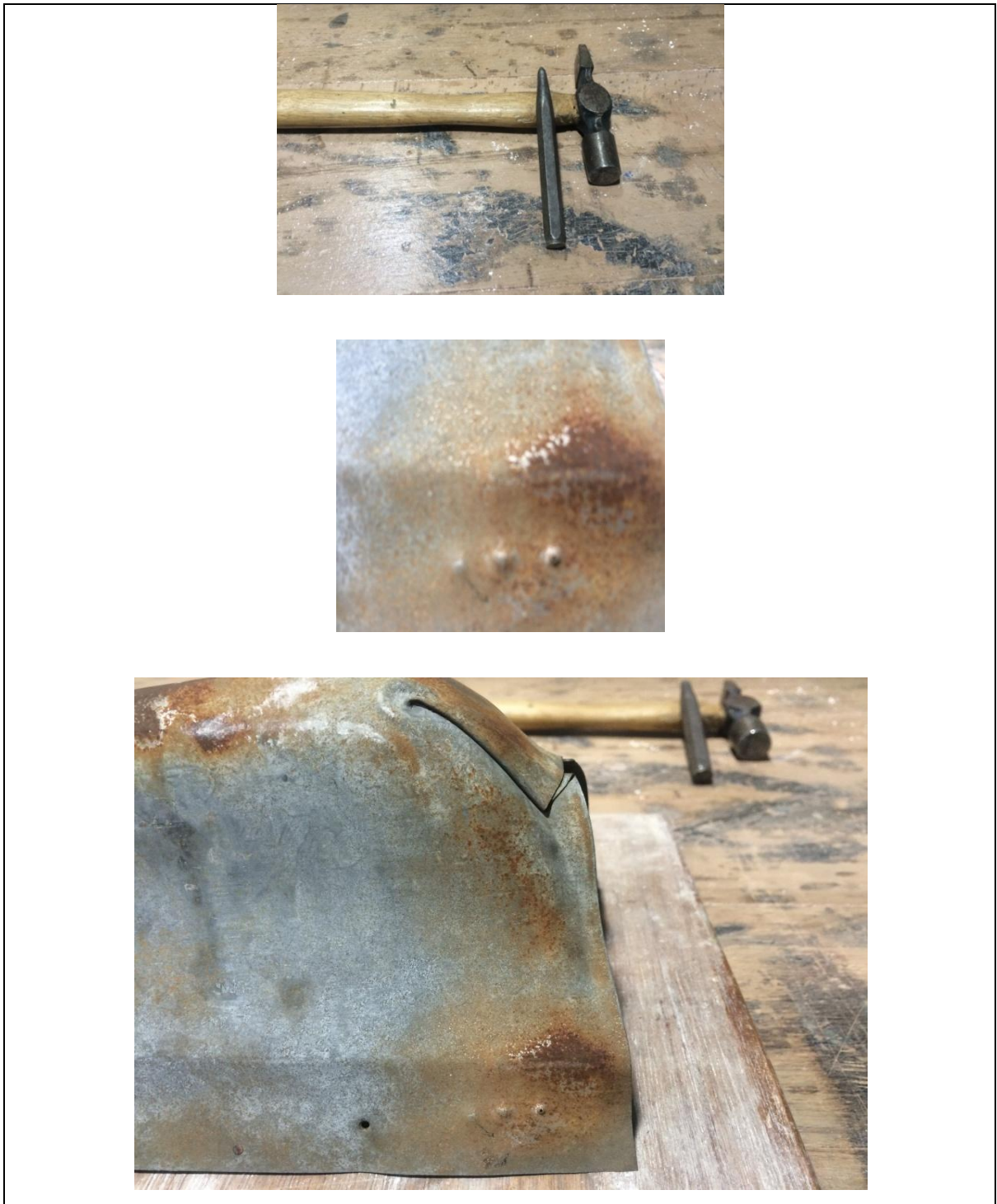
Figure 117 Snyder tin roof hand hammering sample
