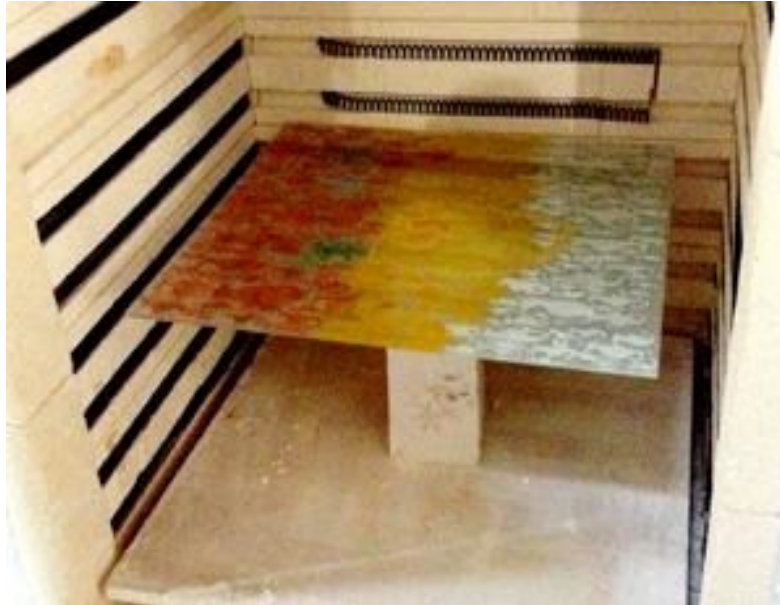
iv) The finished painting glass sheet was put in a kiln.
