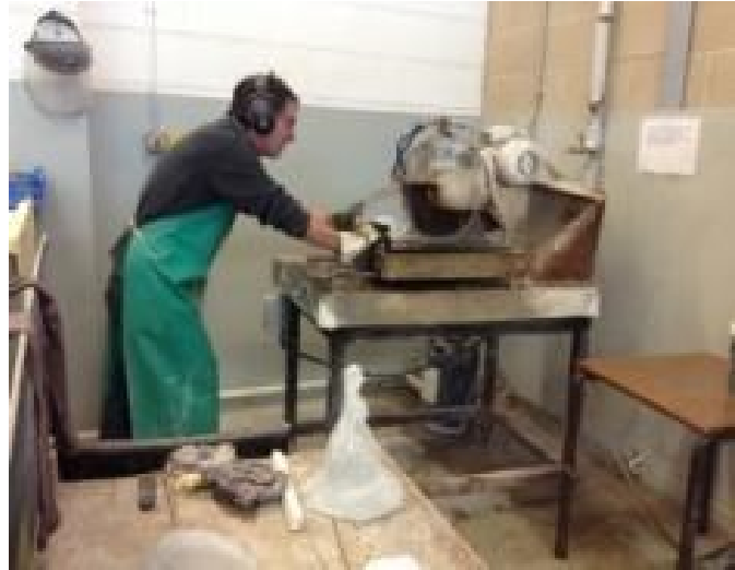
2. Removal of unwanted excess casting
