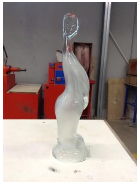
The frosted effect inside after sand-blasting
