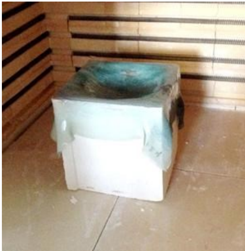
iii) Finished slumped figure in the kiln 30 x 30 x 0.3cm
