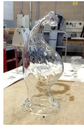
Fig.131: The shape after cut the spare part of the blowing port.
