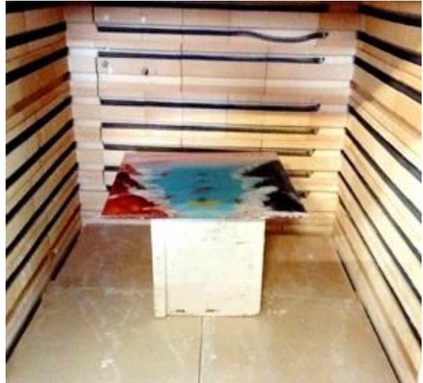
ii) Prepared for slumping
