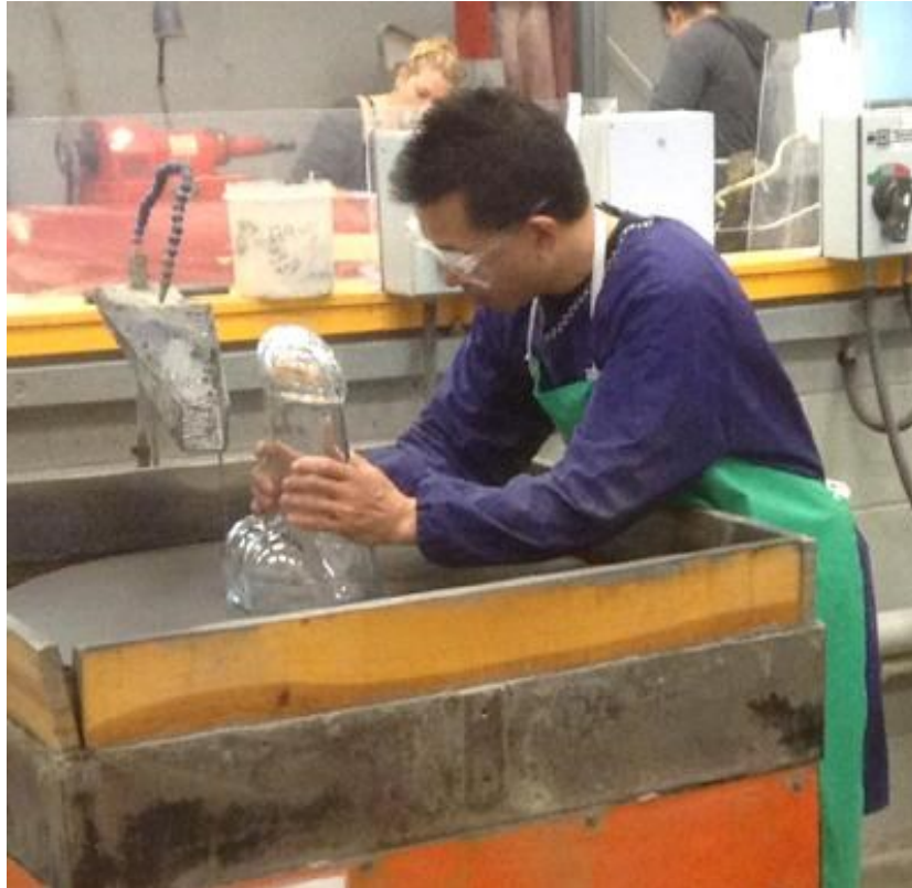
Fig. 142: Polishing the rough bottom of the glass work.
