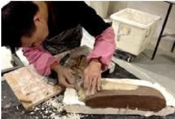
iii) Making a plaster mould
