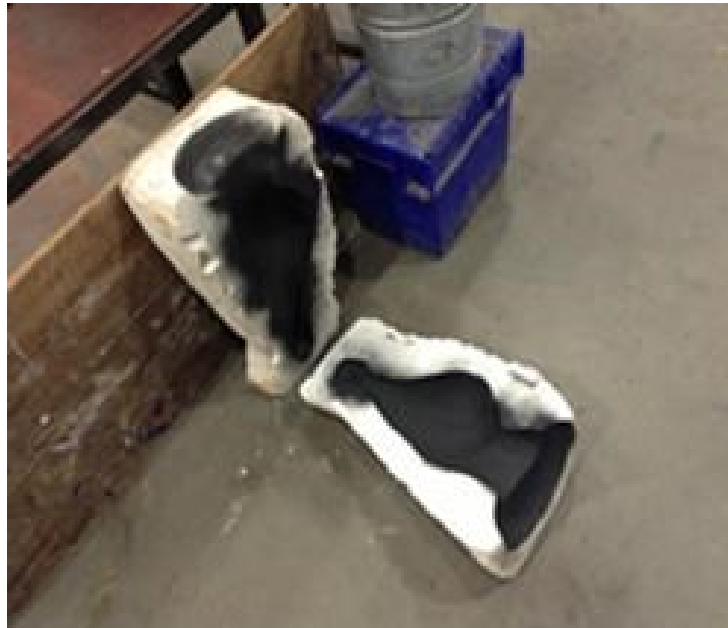
Fig. 128: Sprayed graphite in the „female” plaster mould.
