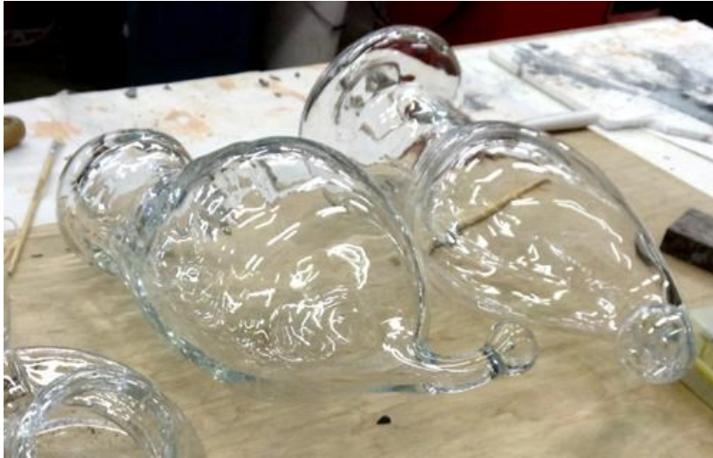
Fig.131: The shape after cut the spare part of the blowing port.
