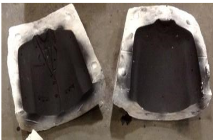
iii) Protecting graphite sprayed onto the inside of the mould.
