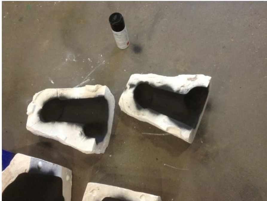
Fig.138: The plaster mould for the blown work Seasons .
