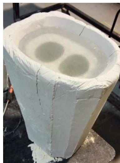
v) The mould after casting full of glass
