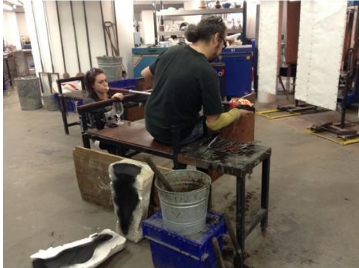
Fig.129: Blowing a bubble according to the size of the mould.
