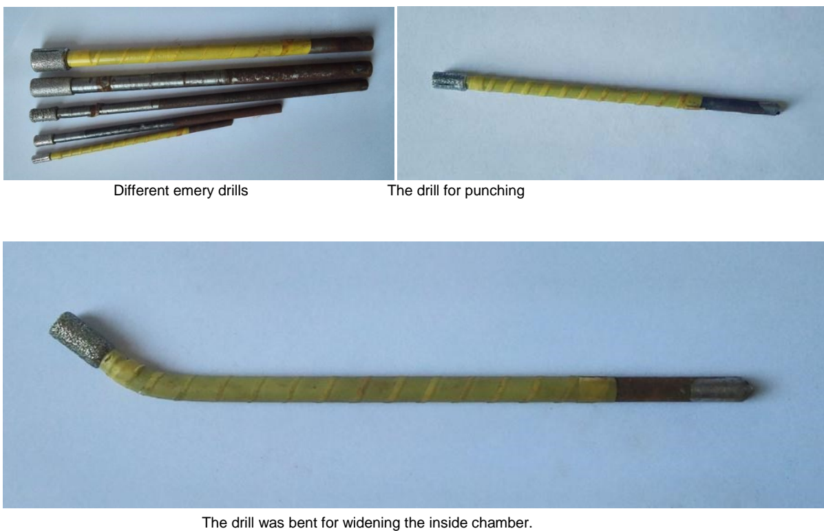
Fig. 110: The different emery drills for punching and widening the inside chamber.
