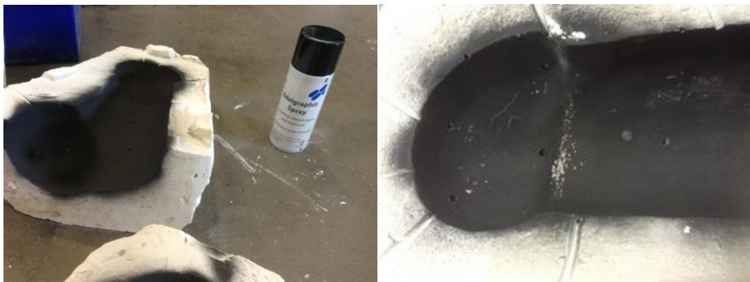
Fig. 139: The mould has been sprayed with graphite fluid.
