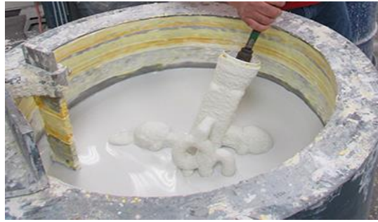
Figure 5: Primary slurry coating [9]
