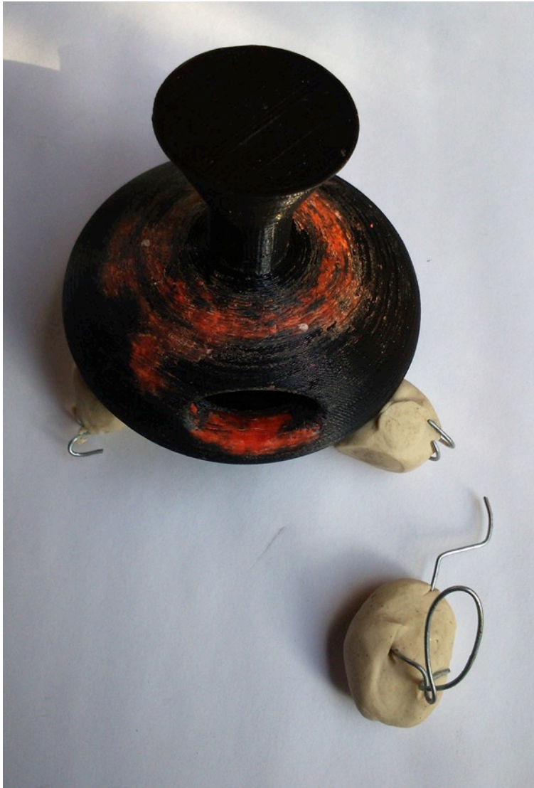
77. Red wax used to fill flaws/defects
