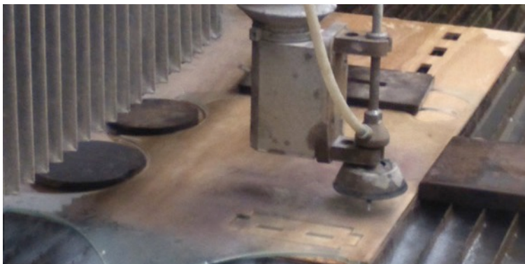
122. Water jet cutting 'bunk bed' stands for ring things
