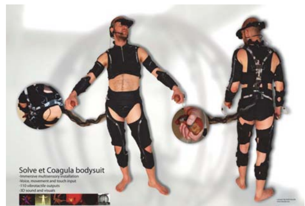
Fig 3. The SeC bodysuit , 1997. The 120 tactile effectors are equally distributed throughout the suit, effectively covering the whole body. The user holds the pressure sensitive devices in each hand. Copyright Stenslie.
