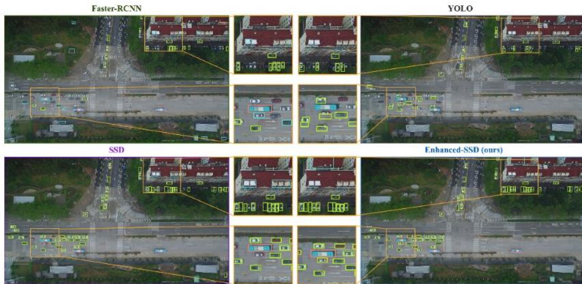
Figure 7: Test 2 Videos results - True positives marked with green boxes. False positives are other colors (Zhu et al 2018).
