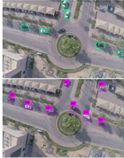
Figure 4: YOLOv3 and Faster R-CNN car detection (Benjdira et al. 2019).
