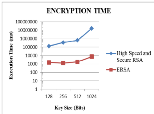
Figure 13: Comparison of encryption Time with different Key Sizes
