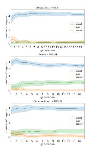
Fig. 9. For each of the three environments, distribution of the number of wheels, joints and sensors over the best robots of each generation. The coloured areas correspond to the confidence interval and the solid curves to the central tendency.
