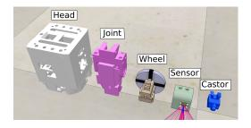
Fig. 3. Active and passive components are used for the experiments shown in this paper. The active components are the wheel, joint and sensor. The passive component is the castor wheel. The head is the central processing unit of the robot.
