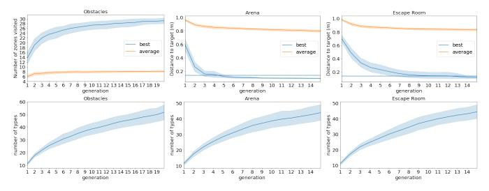
Fig. 7. Plots of three metrics over the generations related to the controllers in the archive. First row: the average and best task-performance. Second row: the number of controllers in the archive. The coloured areas correspond to the confidence interval around the mean.
