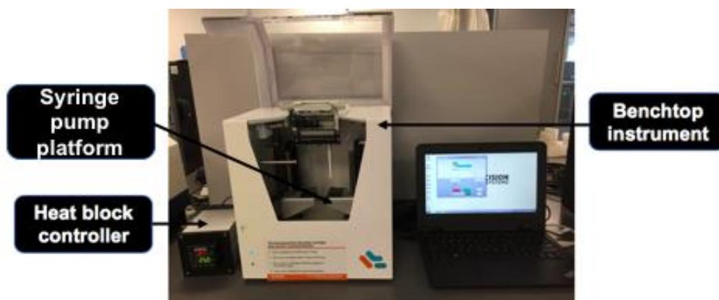
Figure 2-7: NanoAssemblr® Benchtop instrumental system (image was taken in our laboratory, Fleming 107, University of Sunderland).
