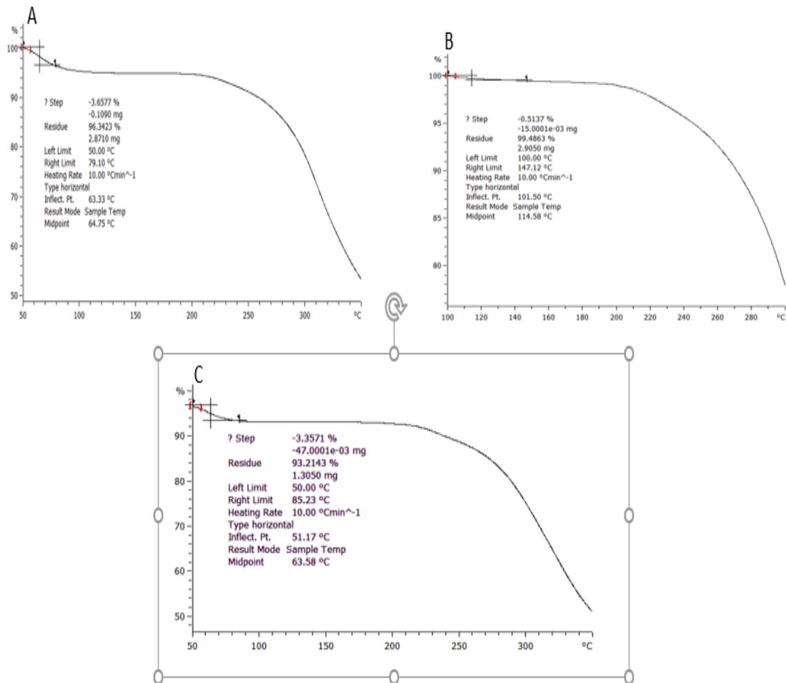
Figure 3.4 TGA curve for (A) 1%w/v unprocessed lysozyme, (B) 1%w/v SD lysozyme, (C) 1%w/v ESD lysozyme
