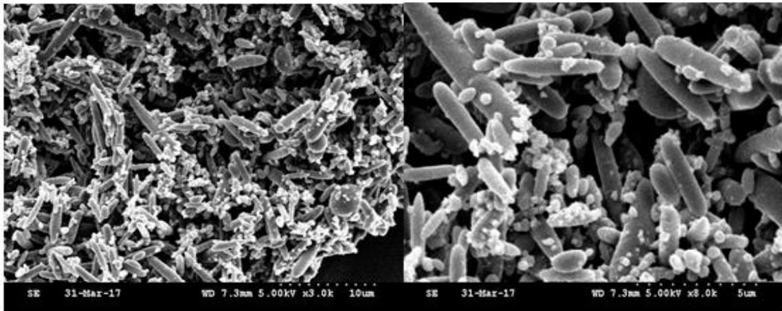
**Figure: 1% Electro sprayed dried Lysozyme with 1% Pluronic**
