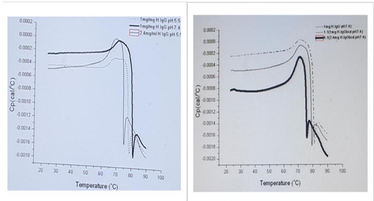
**Figure 5.3** Raw DSC thermogram of human IgG (1 mg/ml;2mg/ml) in a 10-mM sodium citrate, 140mM NaCl buffer, pH 5.5 and 7.4
