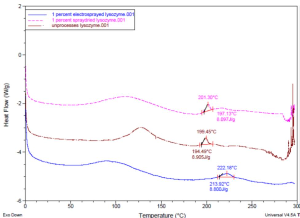
Thermogram showing all unprocessed, spraydried and electro sprayed lysozyme.
