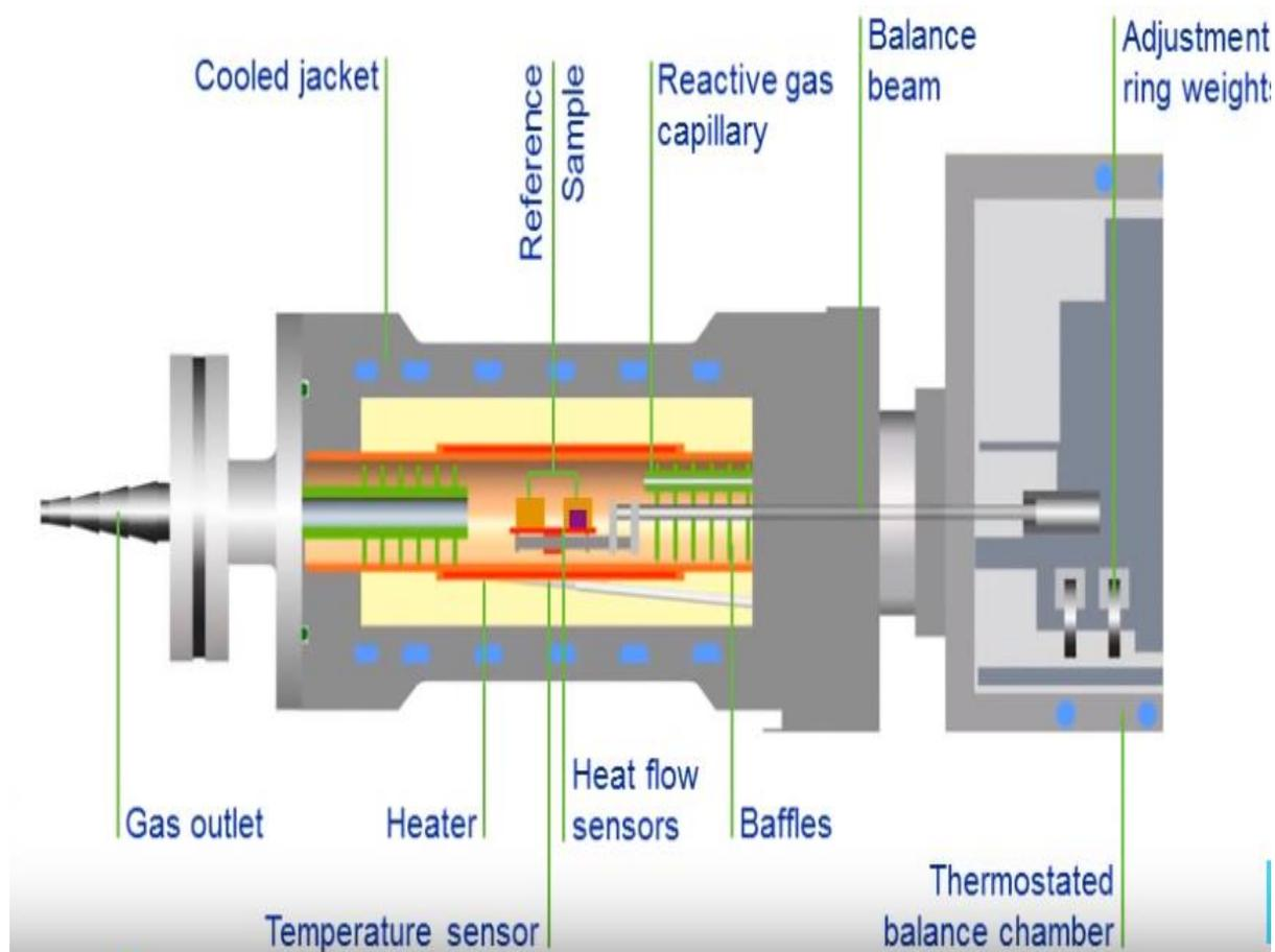
Figure 2.8: illustration of a TGA instrument (Mettler, 2018)
