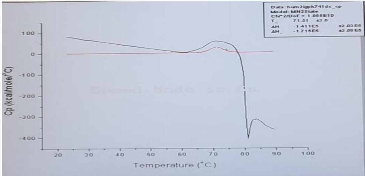
non two state thermogram of human IgG (1 mg/ml) in a 10-mM sodium citrate, 140mM NaCl buffer, pH 7.4
