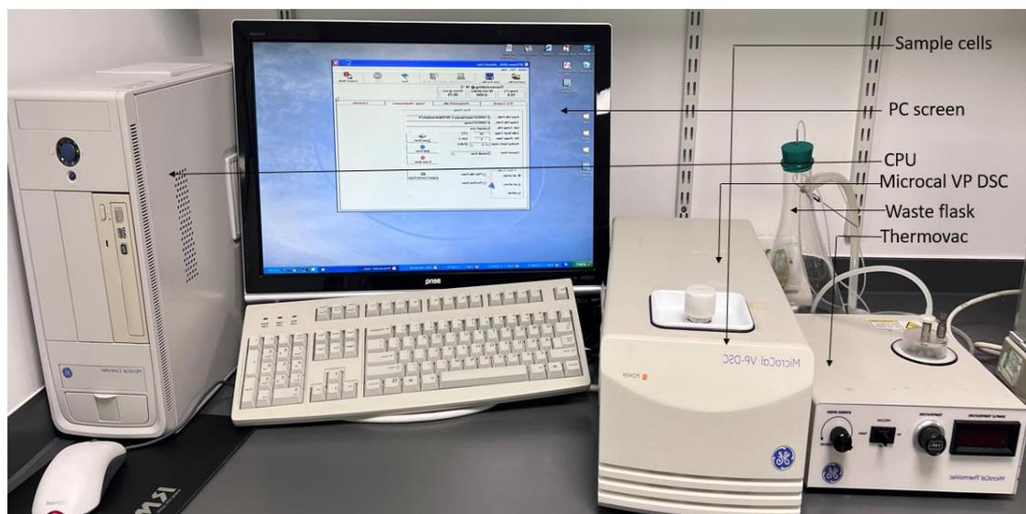
*Figure 2.4 Showing a picture of the high sensitivity differential scanning calorimetry system.*
