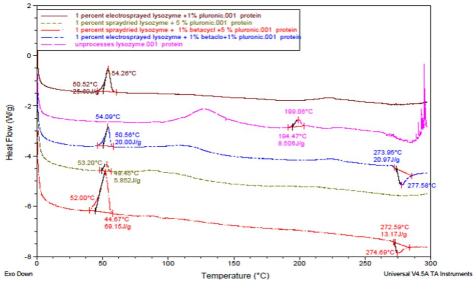
Figures showing thermogram of unprocessed, spray-dried and electrospray lysozyme with excipients
