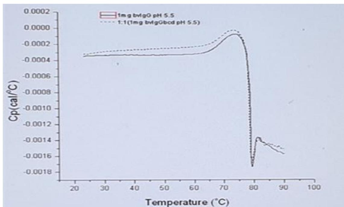
Figure 5.13 Raw data showing little or no effect of denaturation and aggregation temperature of 1mg bovine IgG and 1:1%w/v (1mg) bovine IgG beta cyclodextrin at pH 5.5 where dotted dark line represents 1mg bovine IgG, dotted dark line represents bovine IgG with beta cyclodextrin.
