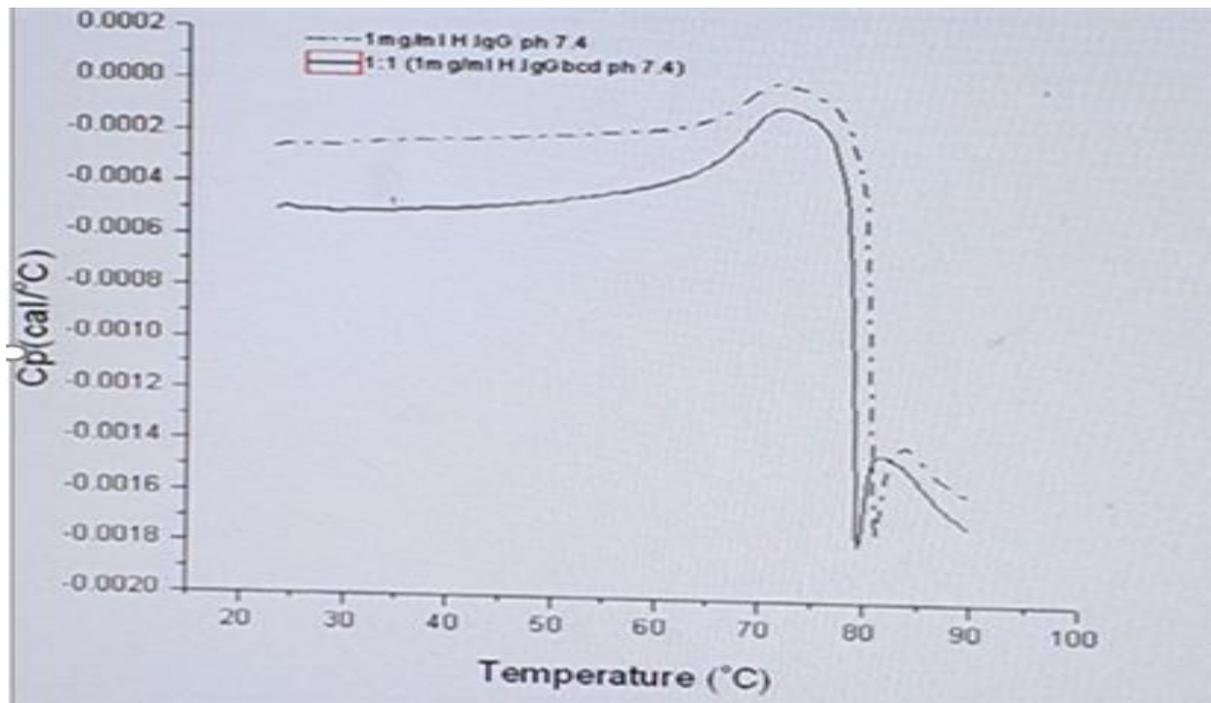
Figure 5.8 Raw data showing reduced aggregation temperature of 1mg/ml human IgG and 1:1%w/v (1mg/ml) of human IgG with beta cyclodextrin at pH 7.4. dark dotted line represents 1mg/ml human IgG; dark line represents 1:1(1mg/ml) IgG with betacyclodextrin.
