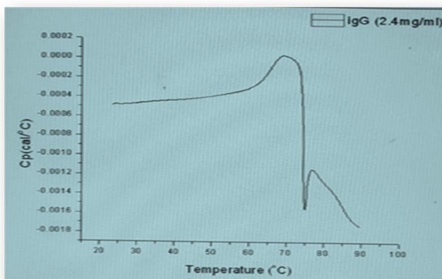
Figure 5.5 DSC thermogram of human IgG (2.4 mg/ml) in a 10-mM sodium citrate, 140mM NaCl buffer, pH 5.5.
