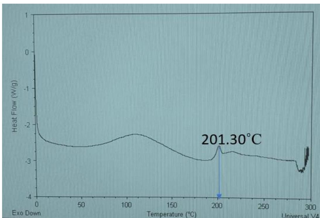
*Figure 3.6: Showing thermal denaturation of spray-dried formulation at a midpoint temperature of 201.30 °C*
