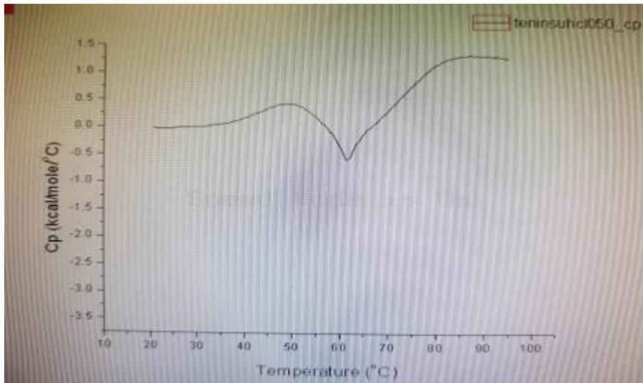
Figure 4.9. Thermogram of showing aggregated insulin in the following conditions: 10mg/ml protein, 0.1M HCl, pH 1.2 at 10°C scan rate
