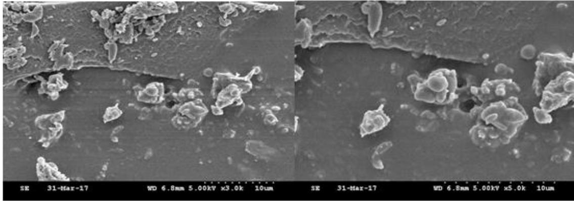
**Figure: 1% Electro sprayed dried Lysozyme with 1% Betacyclodextrin**
