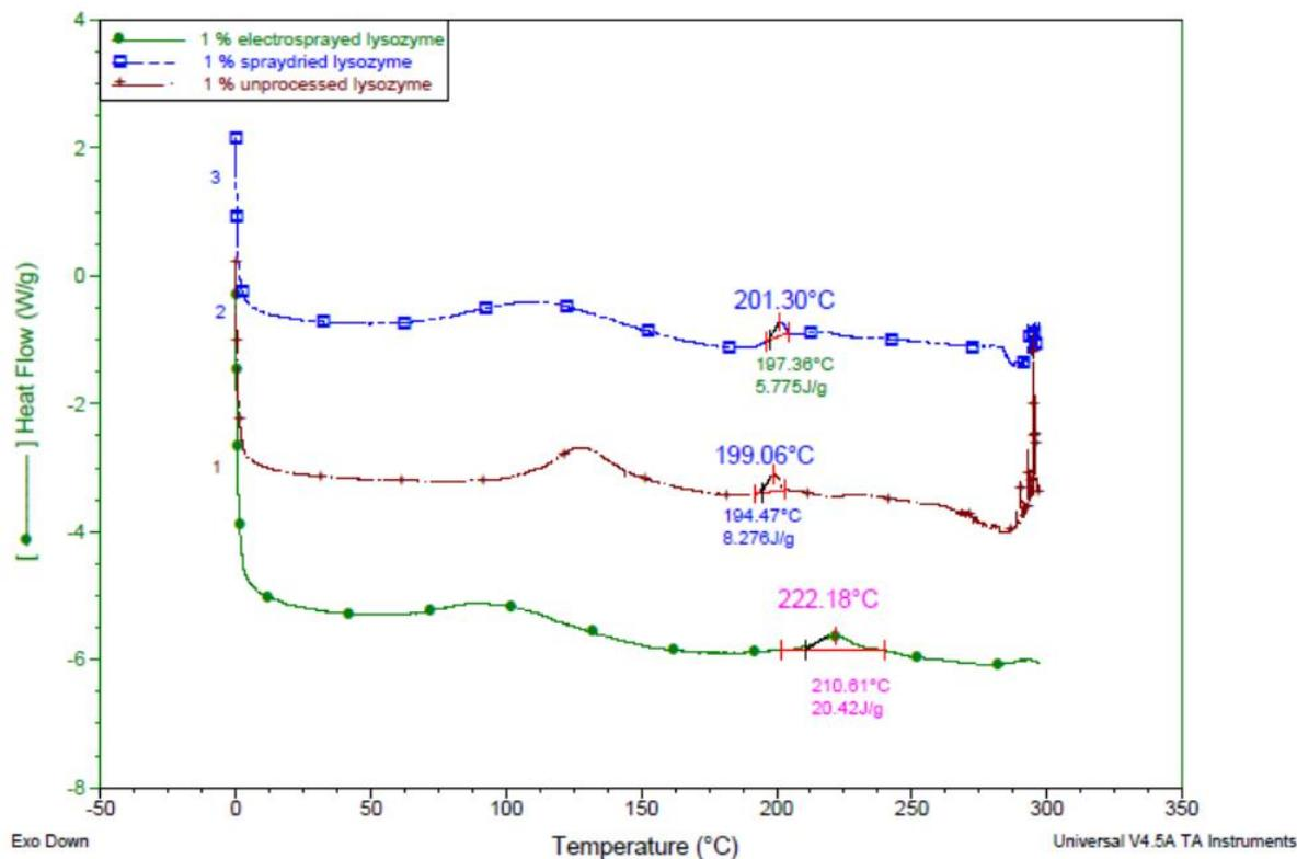
Figure 3.7. DSC thermogram of unprocessed, spray-dried and electrospay lysozyme in the absence of Beta cyclodextrin and Pluronic F-127
