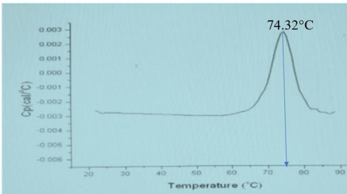
Figure 3.5 Represents a DSC thermogram of unprocessed lysozyme solution. 5mg/ml in phosphate buffered saline at pH 6.24
