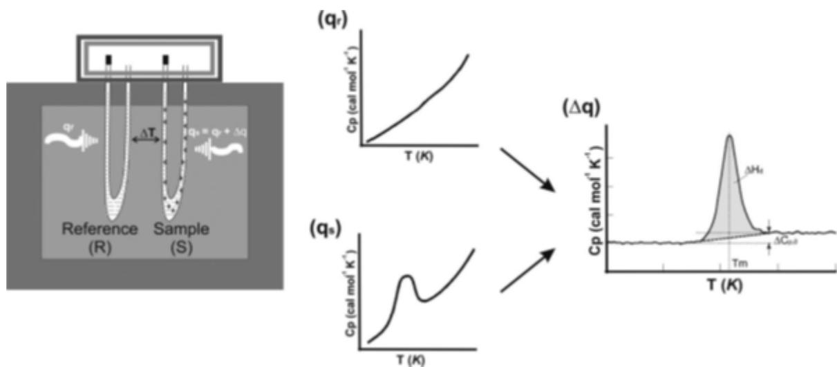
Figure 2.5: illustration of a DSC process (Gill et al., 2010)
