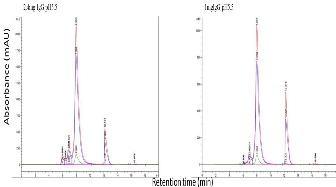
Figure 5.6 Comparison of peak area and retention time for 1mg and 2.4mg concentration at pH 5. n=3
