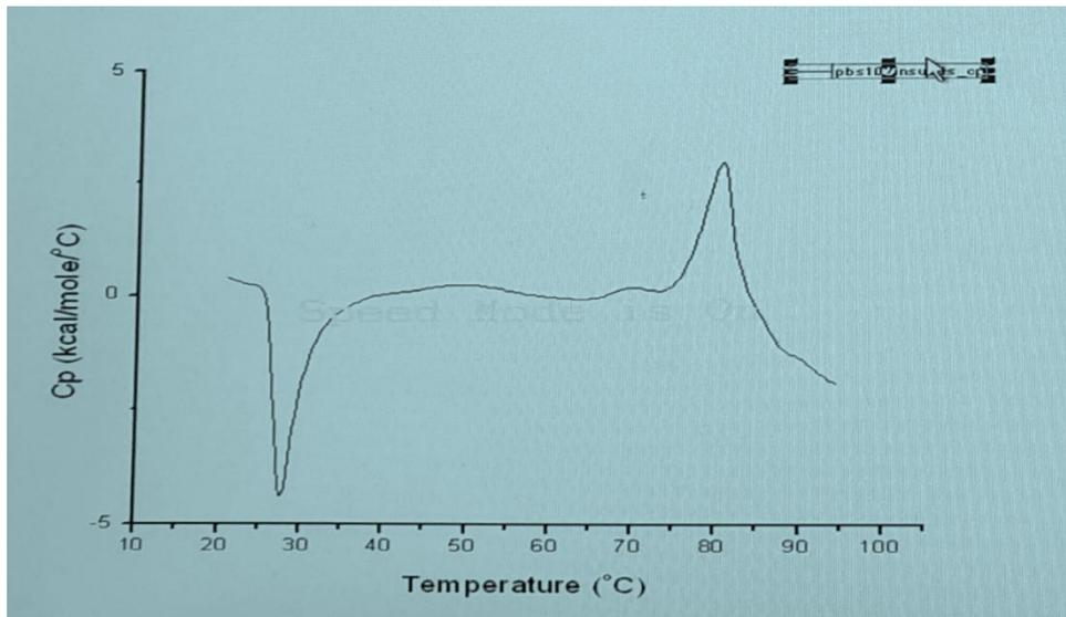
*Figure 4.7 DSC scan representing a 1:1 %w/v insulin containing pluronic F-127 in Phosphate buffered saline pH 7.6.*
