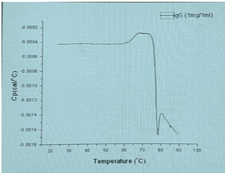
Figure 5.1 DSC thermogram of human IgG (1mg/ml) in a 10-mM sodium citrate, 140mM NaCl buffer, pH 5.5.
