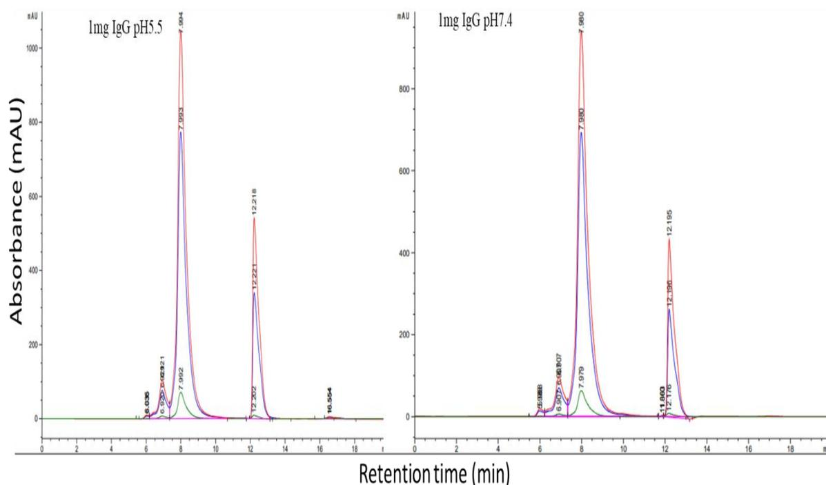
Figure 5.3 Comparison of peak area and retention time of IgG at pH 5.5 and pH 7.4 heated at 60°C. n=3
