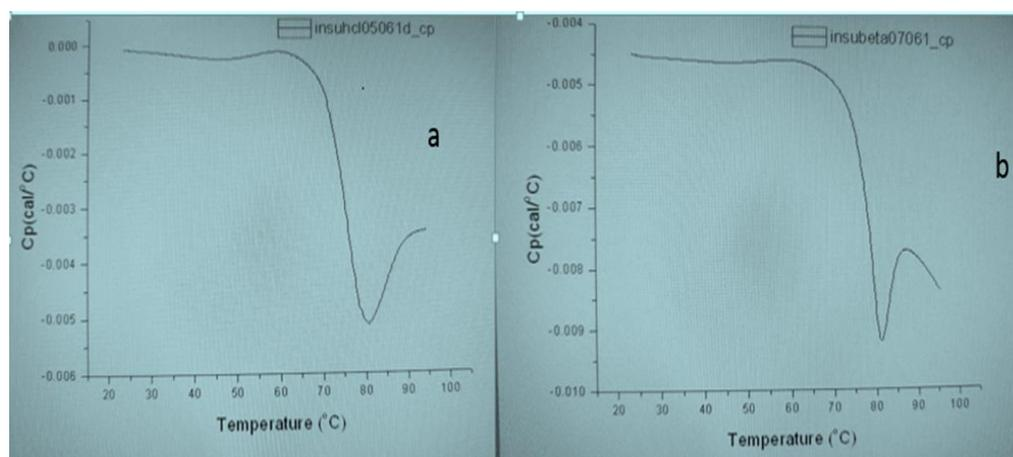
Figure 4.6: Illustration of a thermogram for (a)unprocessed insulin and (b)insulin with beta cyclodextrin insulin in HCl showing the aggregation temperature at 78°C and 79°C at 60°C/hr scan rate.
