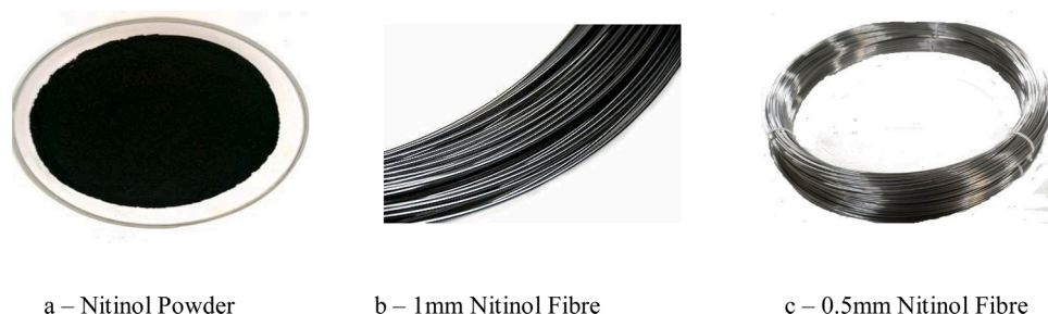
Fig. 1. a – Nitinol Powder Fig 1b – 1 \text{ mm} Nitinol Fibre Fig 1c – 0.5 \text{ mm} Nitinol Fibre.
