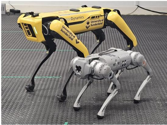
Figure 1: Spot by Boston Dynamics (Bernard) and the Unitree Go1 Edu (Rocky) stood side by side to demonstrate differences in morphology.
