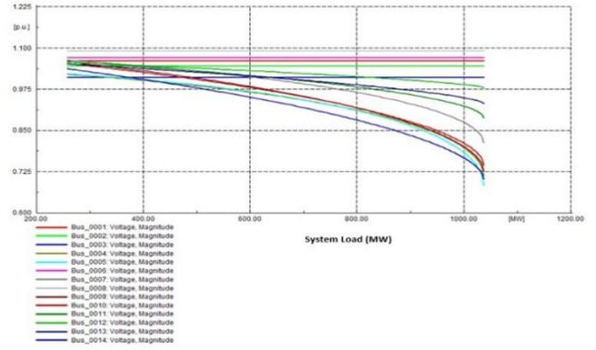
Fig. 6. P-V curves for base case (bus 5 is the critical bus).
