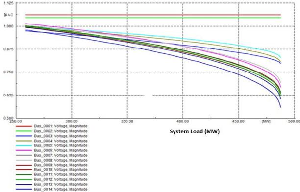
Fig. 2. P-V curves for base case (bus 14 is the critical bus).
