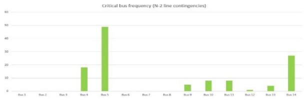
Fig. 9. Bar graph showing that Bus 5 is the critical bus for (N-2) line contingencies.
