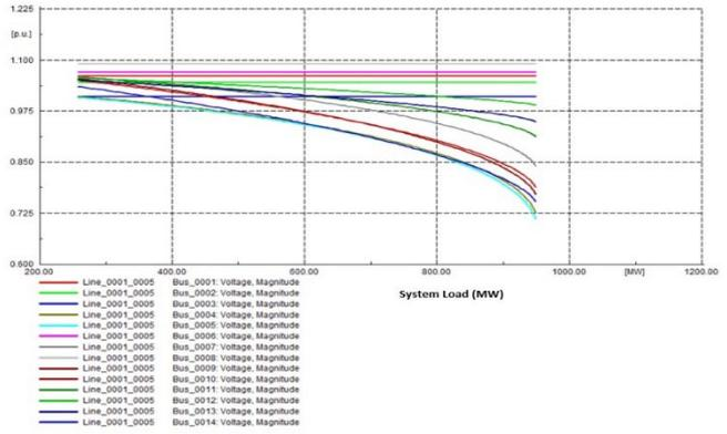
Fig. 7. P-V curves for Line 1-5 contingency (bus 5 is the critical bus).
