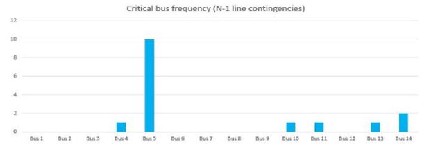
Fig. 8. Bar graph showing that Bus 5 is the critical bus for (N-1) line contingencies.
