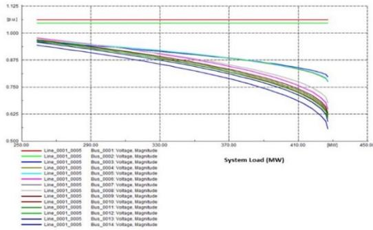
Fig. 3. P-V curves for Line 1-5 contingency (bus 14 is the critical bus).
