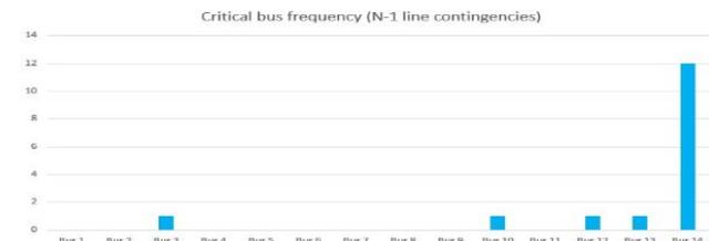
Fig. 4. Bar graph showing that Bus 14 is the critical bus for (N-1) line contingencies.
