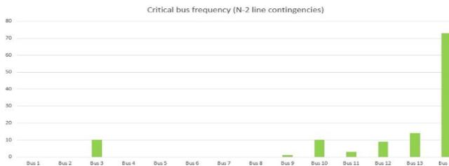
Fig. 5. Bar graph showing that Bus 14 is the critical bus for (N-2) line contingencies.
