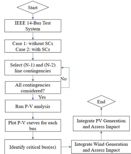
Fig. 1. Computation procedure.
