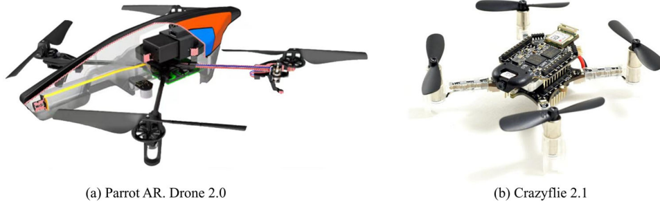
FIGURE 14 | Examples of UAV platforms. (a) Parrot AR. Drone 2.0 (b) Crazyflie 2.1. [Color figure can be viewed at wileyonlinelibrary.com ]
