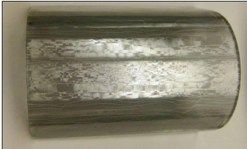
Figure 5.48 4mm ST150, post-fired at 775°C, bending test.
