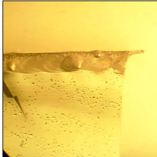
Figure 4.7 6mm K, post-fired, edge view showing overhang.
