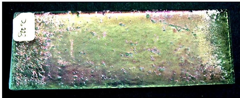
Figure 3.38 4mm K, post-fired at 800°C, showing bubble formation.
