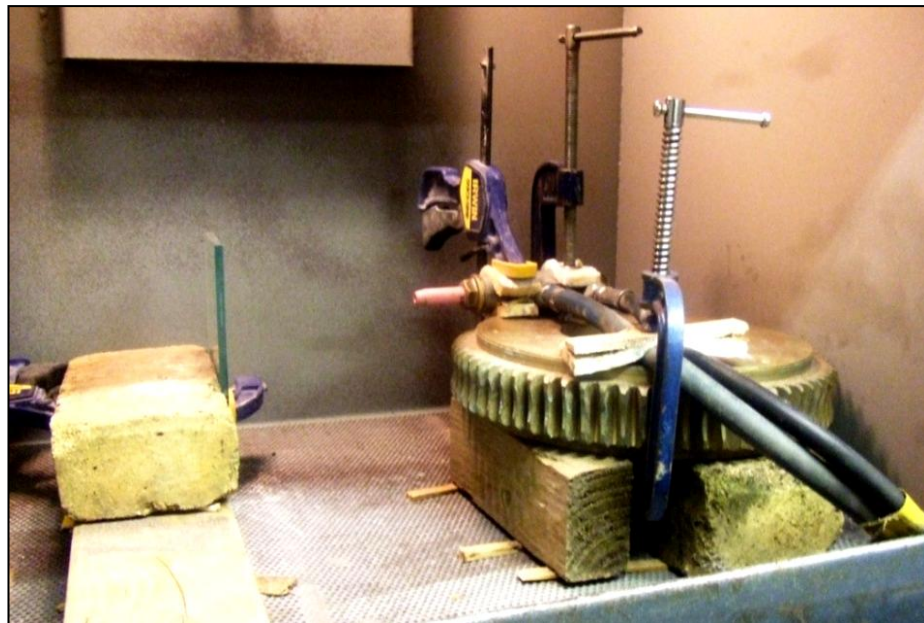
Figure 5.24 Arrangement for sandblasting grit study.
