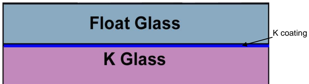
Figure 3.1 Fused Glass format of fusing position of K and float glass.
