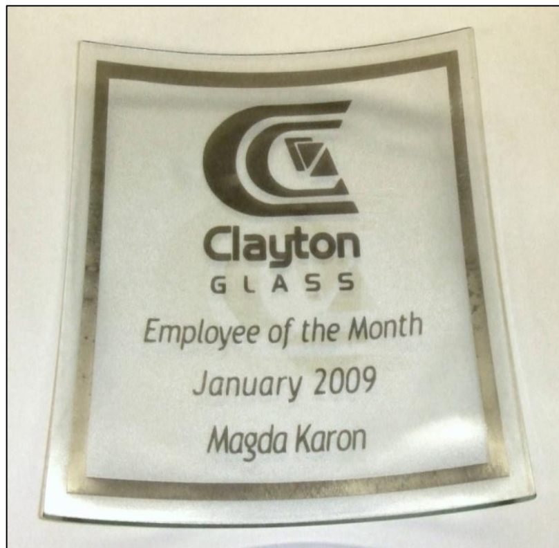
Figure 5.45 4mm ST150, post-fired at 775°C.
