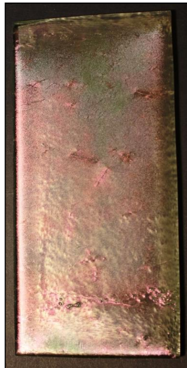
Figure 3.54 4mm K, post-fired at 775°C with slow schedule 2, showing no patches.
