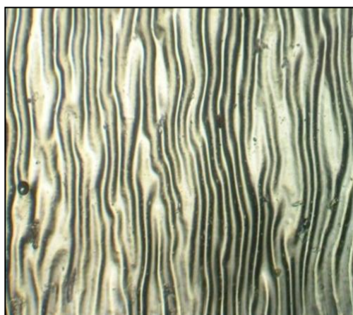
Figure 4.3 6mm K, post-fired surface, plan view showing ripples.
