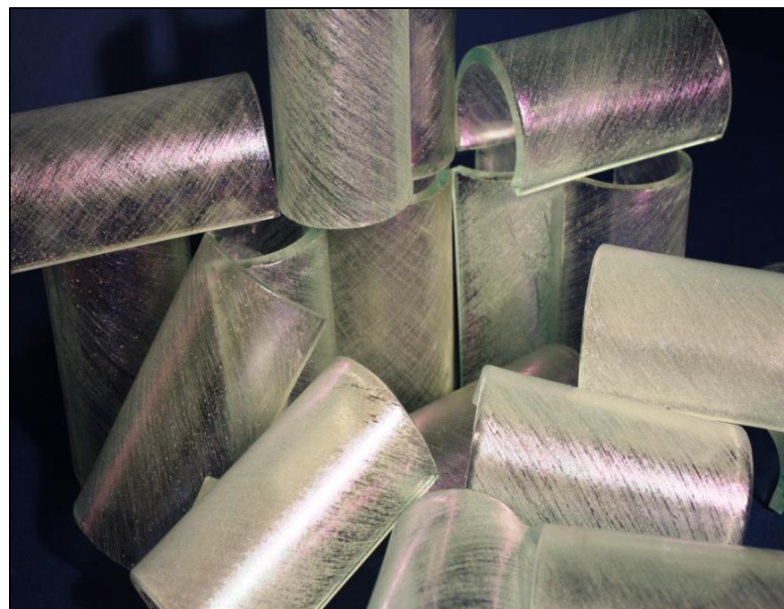
Figure 6.17 4mm K and 6mm K, curved abrasion test pieces.
