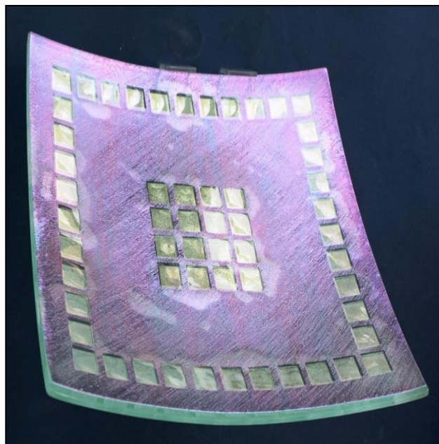
Figure 6.27 'Plate 9', Test plate, 4mm K and 4mm float, Mirror Gap Technique with scored upper layer.
