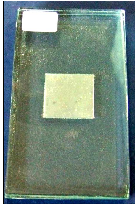
Figure 5.32 Third sandblasted gap showing gold colouration.
