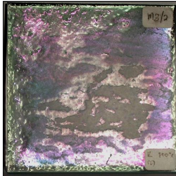
Figure 1.3 4mm K Glass, post-fired showing iridescent colouration to the surface.
