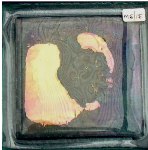
Figure 3.70 4mm K between 6mm float, post-fired at 800°C, showing gold colouration.
