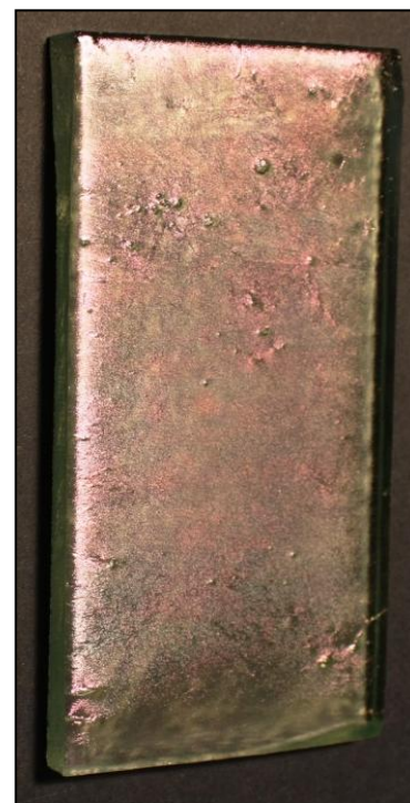
Figure 3.55 6mm K, post-fired at 775°C with slow schedule 2, showing no patches.
