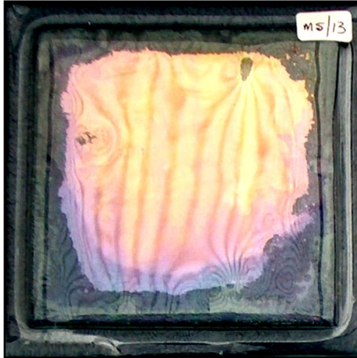
Figure 3.68 4mm K between 3mm float, post-fired at 800°C, showing gold colouration.
