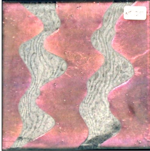
Figure 3.48 4mm K, post fired at 800°C, sandblasted, showing iridescence differences.
