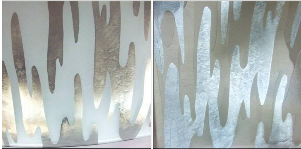
Figure 5.46 ST150 solar coated side, post-fired at 775°C.
