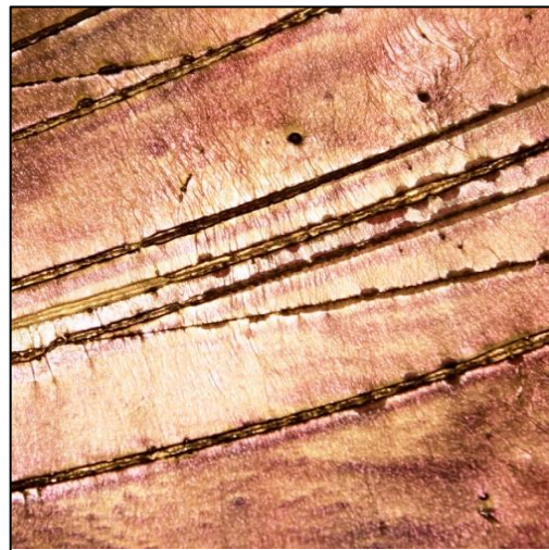
Figure 3.42 4mm K, post-fired at 800°C, photograph of scored surface ripples.
