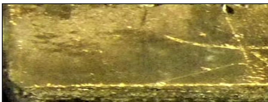
Figure 3.74 4mm K, post-fired at 775°C, fused cut open sample showing gold iridescence.
