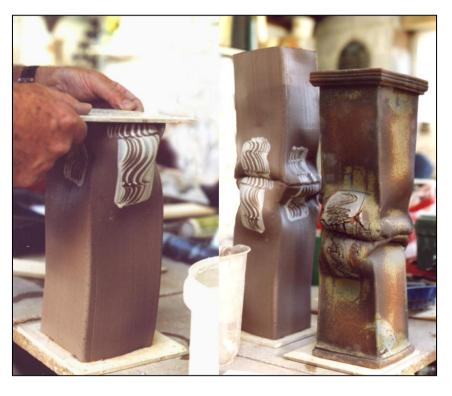
Figure 66: Stages in making an extruded pot and the finished pot [Photography: Carol Metcalfe]
