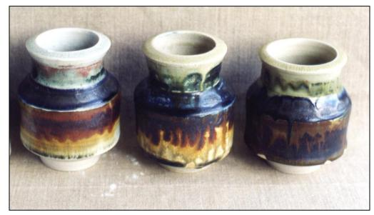
Figure 61: Test pots using cherry, pear & beech ash glazes cause bands of copper, cobalt & iron oxides to collapse and run. The colours developed also differ.
