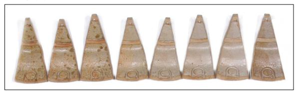
Again the layout of this method allows for recipes with any ash content up to and including 100% and adjustments to the graduations between the tests could be introduced, if required, offering similar versatility to the triaxial blend. Equally, extra tests could be introduced within a specific range, making the line blend a simple but effective method of exploration, when combinations of only two ingredients are required.
