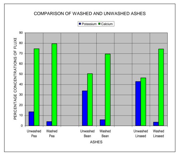
Figure 24: Chart showing the effect of washing on the flux content of ash
