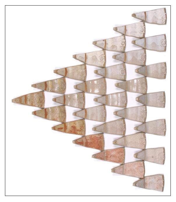
Figure 124: Test set 2: Unwashed bean ash recipes UB2.1 – UB2.28 on Camberwell clay [Photography: David Williams]
