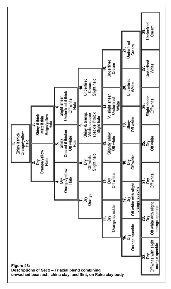
A number of the tiles were under fired, the glaze not having melted at the firing temperature used. At higher temperatures these recipes might well produce useful glazes; however, it is outside the scope of this research to investigate this possibility, the aim being to develop glazes for the lower stoneware temperatures.
