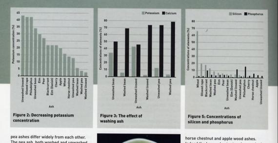
pea ashes differ widely from each other. The pea ash, both washed and unwashed, has levels of calcium similar to the wood ash from horse chestnut, whilst the unwashed bean ash contains much less. Instead it has a high concentration of potassium.
