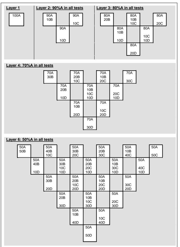
In all, 11 layers are required to give graduations of 10% by weight between tests. Whilst this is a very comprehensive method it does involve a very large
