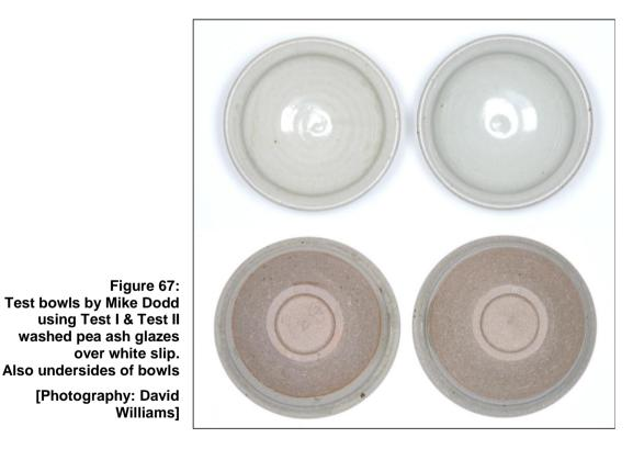
The test bowls produced by Dodd, using the glazes in Table 20, are shown in Figure 67 above. The very pale greenish and blue green colours developed are typical of reduction-fired glazes containing small amounts of iron, which the analyses showed to be present in the pea ash. Both glazes were considered
