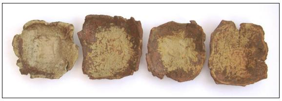
Figure 27: Bean ash test bowls arranged from Left to Right in increasing potassium content
