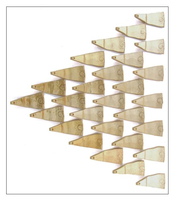
Figure 127: Test set 2: Unwashed pea ash recipes UP2.1 – UP2.28 on Smooth Buff clay [Photography: Carol Metcalfe]
