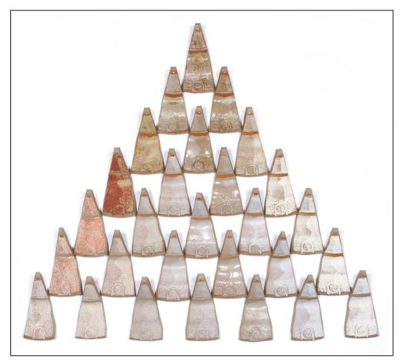
Figure 50: Example of a triaxial blend of test tiles using unwashed bean ash on Smooth Buff stoneware clay body.
