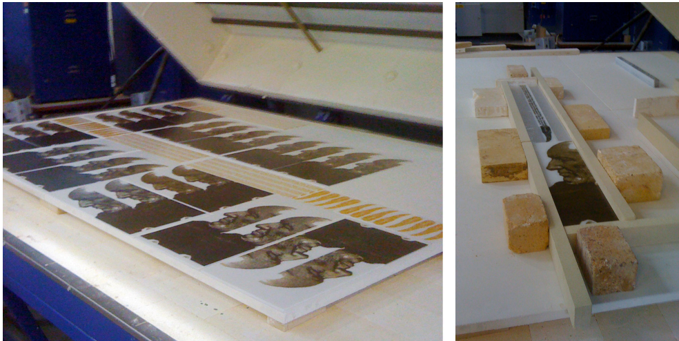
Figure 61 Process: screenprinted multiple glass sheets (left), kiln fusing setup (right)
