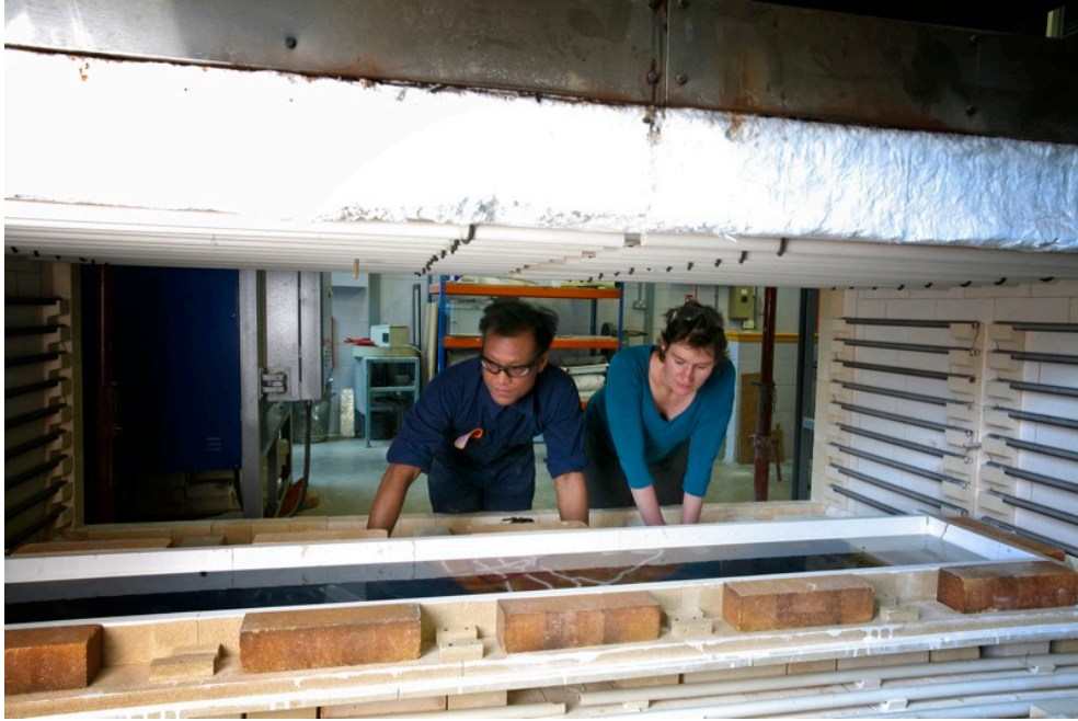
Figure 85 Jeffrey Sarmiento and Inge Panneels inspecting large kiln setup, showing brick and 'sled' support system
