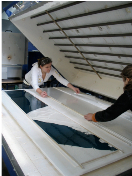
Figure 84 Fusing puzzled glass elements together in kiln
