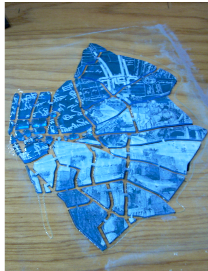
Figure 81 Waterjet cutting section of white glass road map
