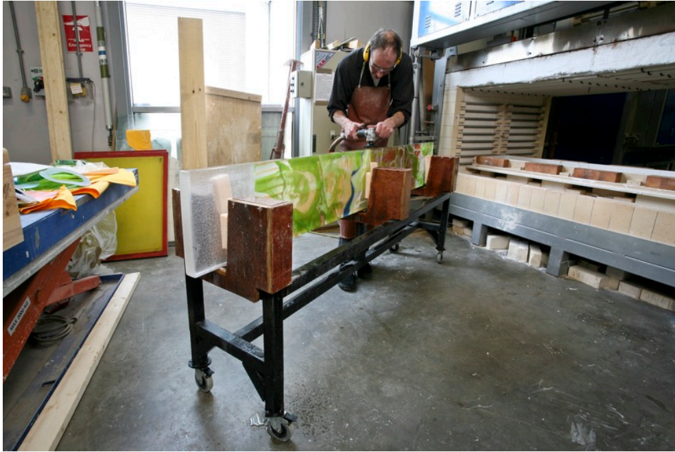
Figure 86 Column 6 of Liverpool Map on cold polishing jig
