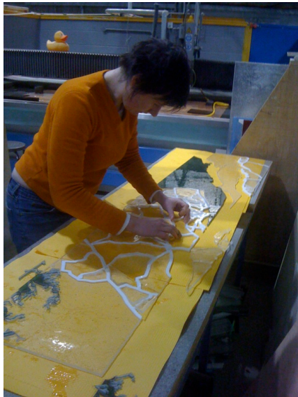
Figure 83 Inge Panneels puzzles together waterjet cut coloured glass components prior to fusing
