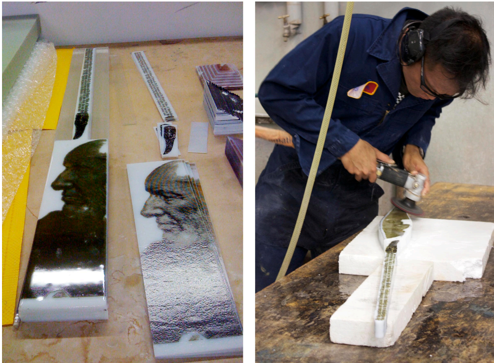
Figure 62 Process: fully fused glass, shown with stack of parts (left), grinding glass into final shape (right)
