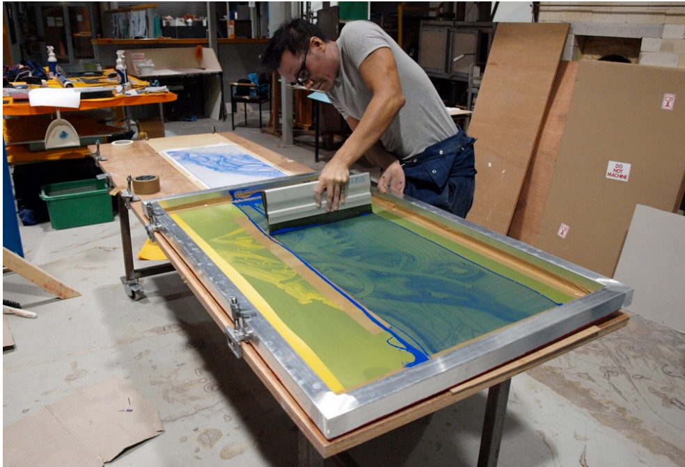
Figure 79 Jeffrey Sarmiento screenprinting enamels onto long sheet of glass
