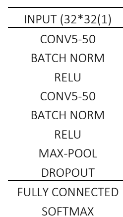
Figure 3: CNN Architecture with 2 convolutional and 2 max-pool layers.
