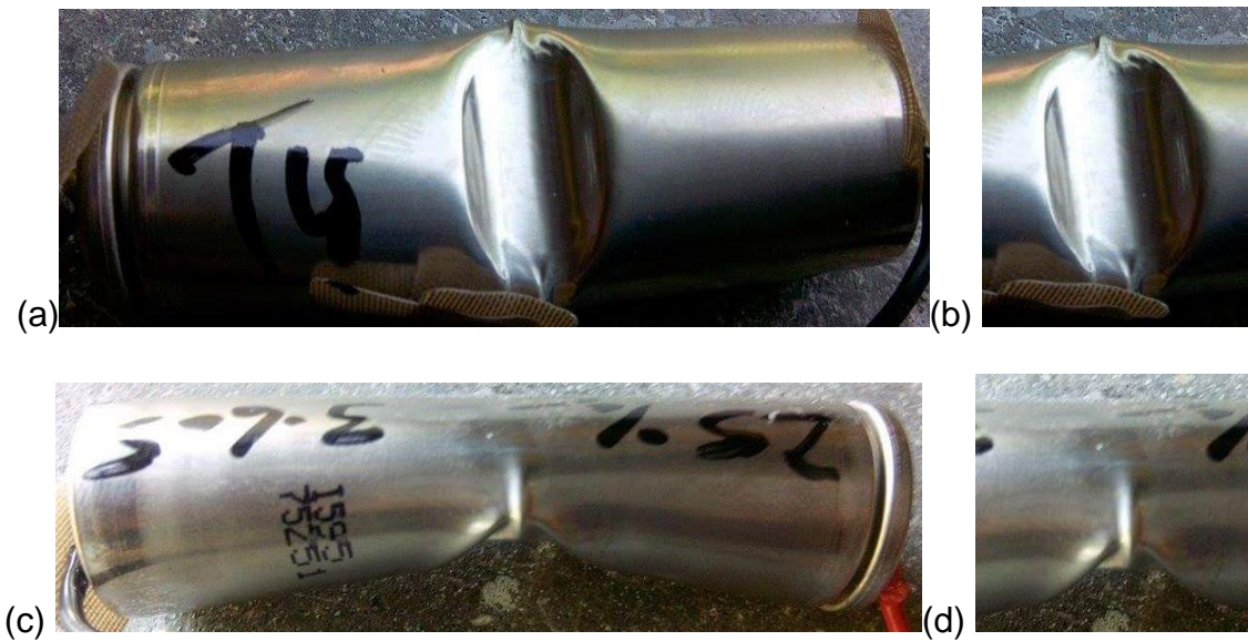
Figure 4.7: Cell physical changes, (a) Top view, (b) buckling of top, (c) side view, (d) buckling of side
