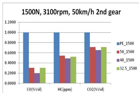
Figure 2: Results for different fuel mixes (3100RPM)
