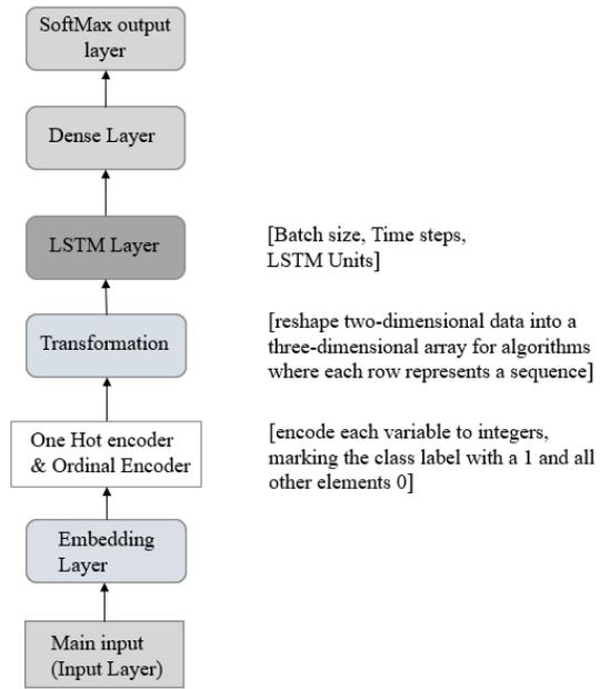
Fig. 1 The Proposed System Architecture with represent each Layer
