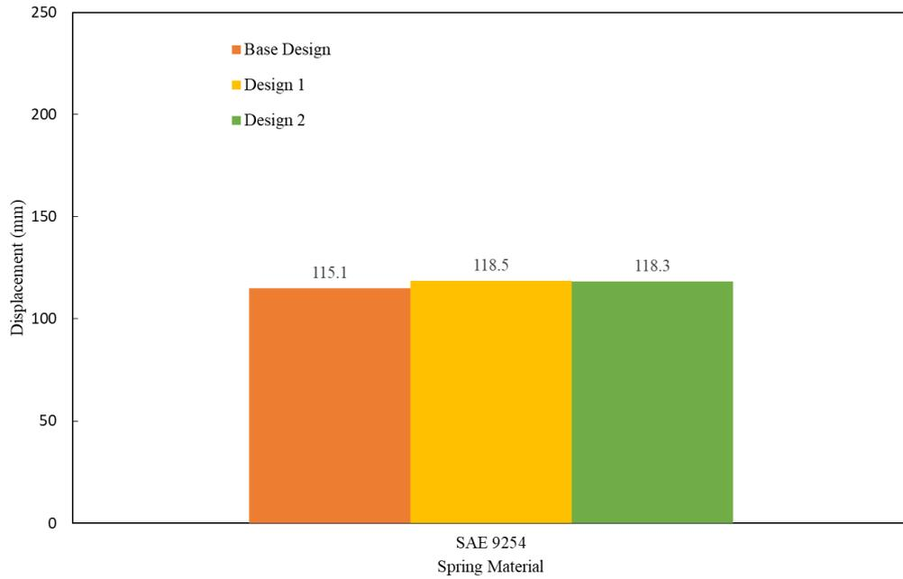
Figure 8: Maximum displacement found in each model.
