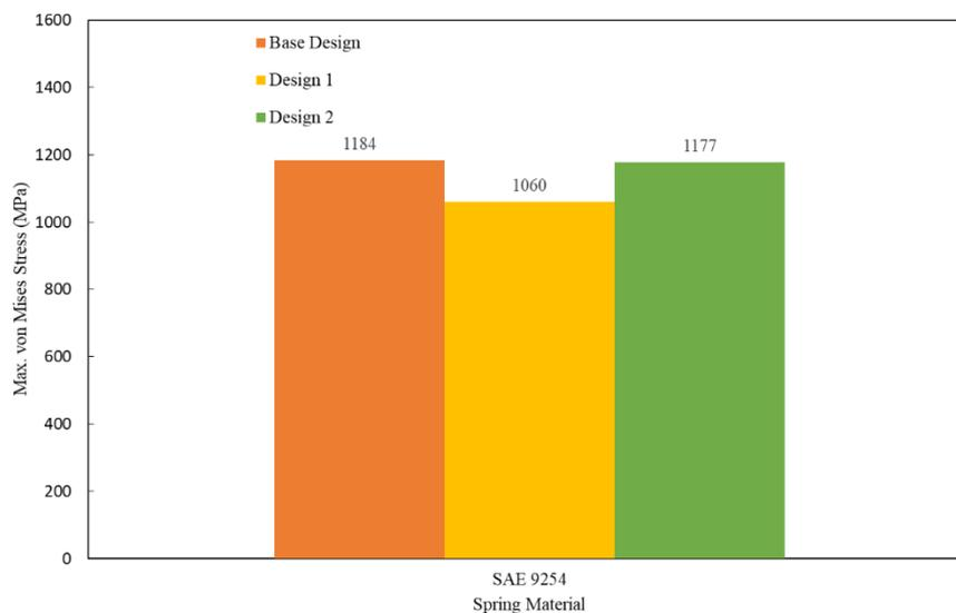
Figure 7: Maximum von Mises Stress found in each model.
