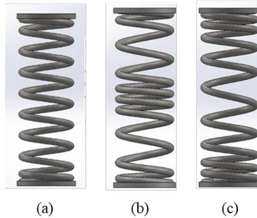
Figure 2: Shows the coils arrangements for all three designs (a) Base Design, (b) Design-1 with smaller pitch at the centre, (c) Design-2 with increasingly larger pitch towards the centre of the spring.
