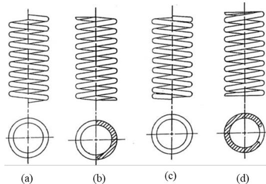
Figure 1: End Types of Compression Springs; (a) Plain Ends, (b) Plain Ends Ground (c) Squared Ends (d) Squared and Ground Ends [8].
