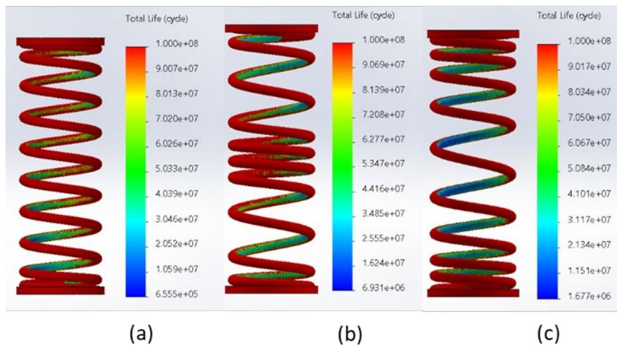
Figure 6: Fatigue life (cycles) for all three models using SAE 9254 material type (a) Base Design, (b) Design-1 and (c) Design-2.
