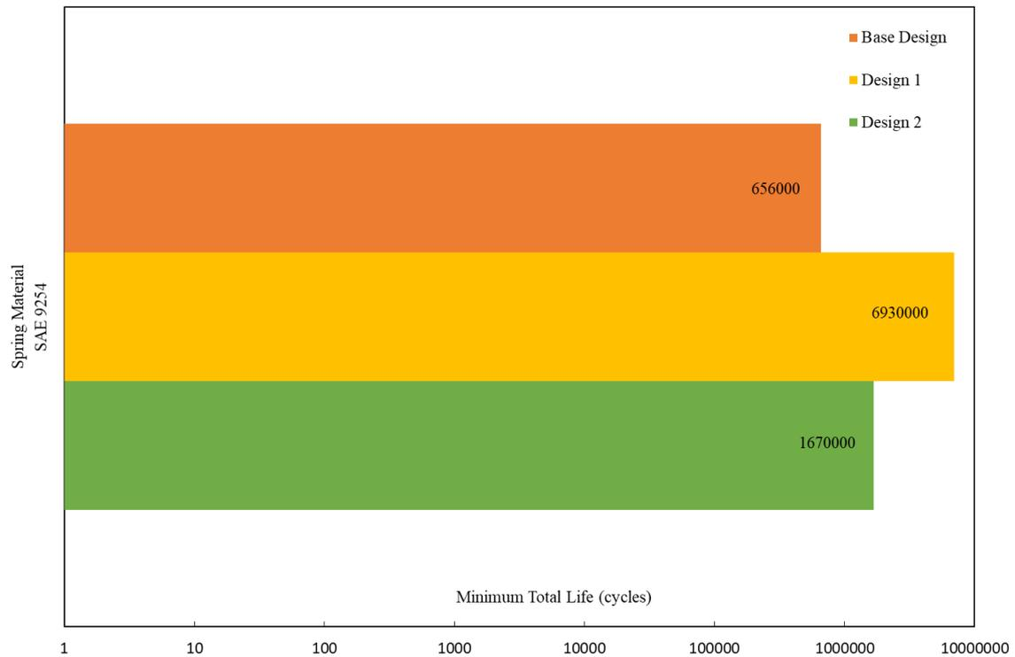
Figure 9: Minimum Total Life (cycles) found in each model.
