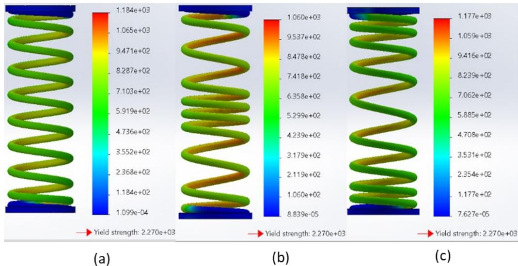
Figure 4: von Mises stress distribution (in MPa) for all three models using SAE 9254 material type (a) Base Design, (b) Design-1 and (c) Design-2.
