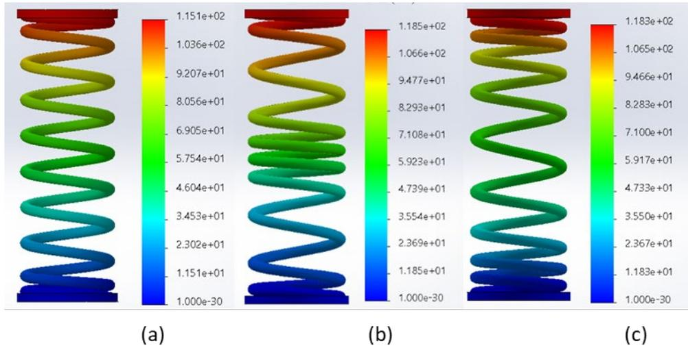
Figure 5: Static Displacement (in mm) for all three models using SAE 9254 material type (a) Base Design, (b) Design-1 and (c) Design-2.
