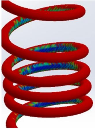
Figure 10: Critical location on Design-1
