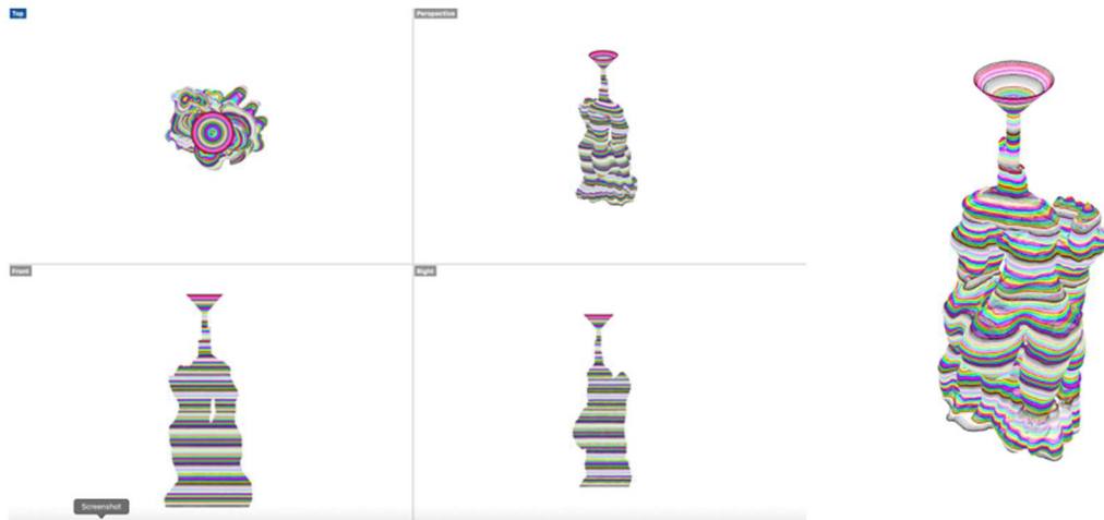
Figure 48; Using the plug-in grasshopper I was able to divide the 'Figure with funnel' mesh into a series of layered curves, Theo Harper, 2019
