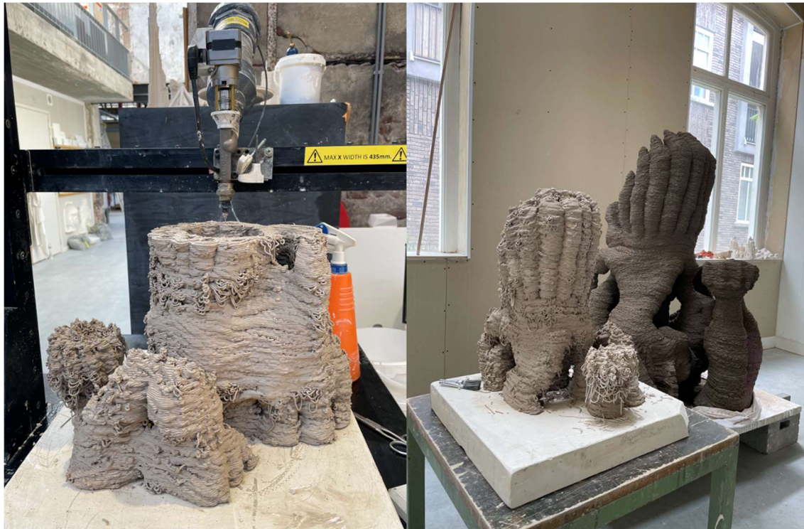
Figure 83; The top half of the digital model being printed in clay using the Lutum 3d printer, EKWC 2021
