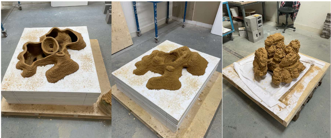
Figure 87; HPC back into the polystyrene mould, EKWC, 2021
