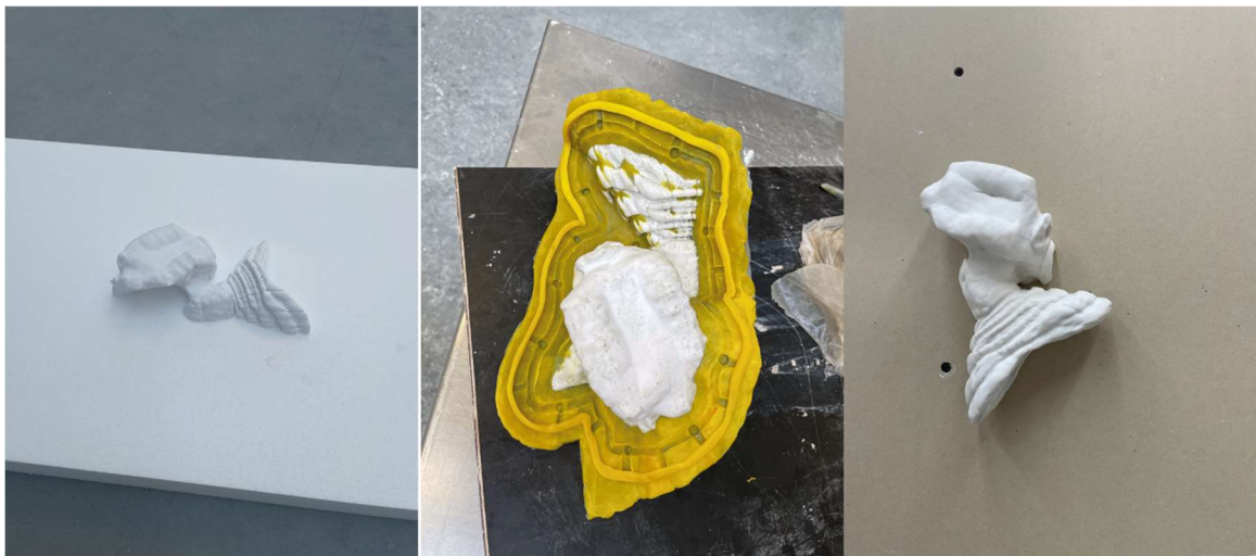
Figure 91; from left, PLA 3D print, mould making, porcelain reproduction, EKWC, 2021
