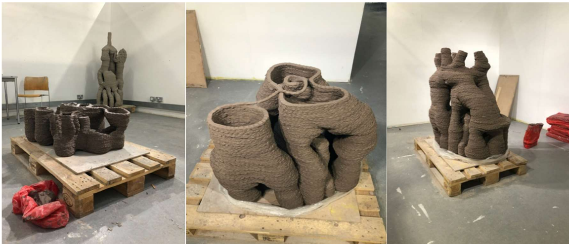
Figure 55; Built in the same way as 'funnel' but using a different clay type (crank). 3d scanning as the HPC form emerges. Theo Harper, 2020
