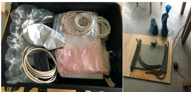
Figure 208; the magnetic movement tracking system (Polhemus)
