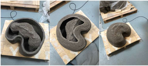
Figure 8; the emergent clay form in stages of completion, closing off the tracker from sight, testing its ability to track through thick clay walls
