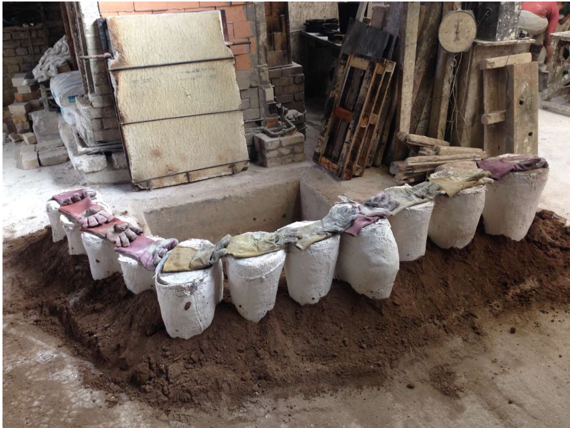
Figure 117; Arch Bronze, ludo moulds after being in the kiln (still warm), with foundry gloves, 2015
