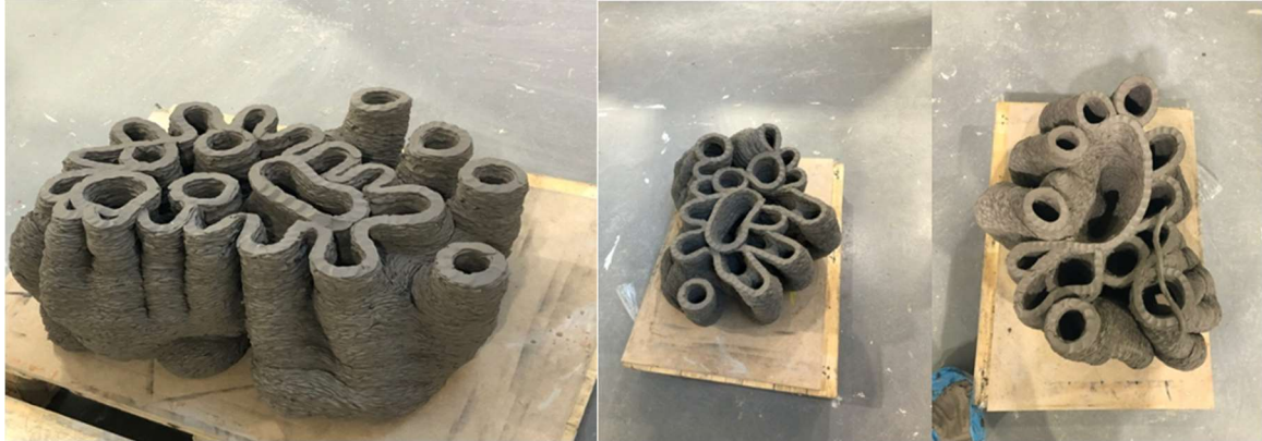
Figure 42; The base beginning with a drawing on the wooden pallet, the layers are built up until it is flipped upside down so that the material can establish a closer relationship with the ground. Sunderland University, Theo Harper, 2019
