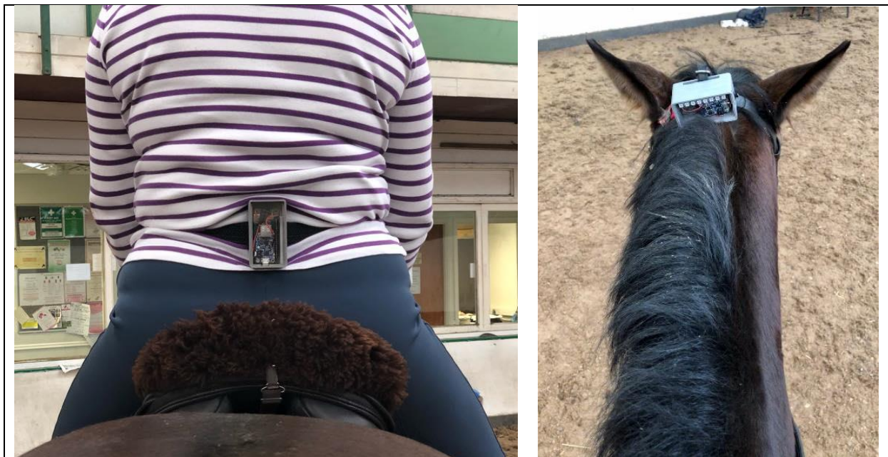
Figure 5.11. IMU Rider(left) and LED Horse (right) devices in position.
