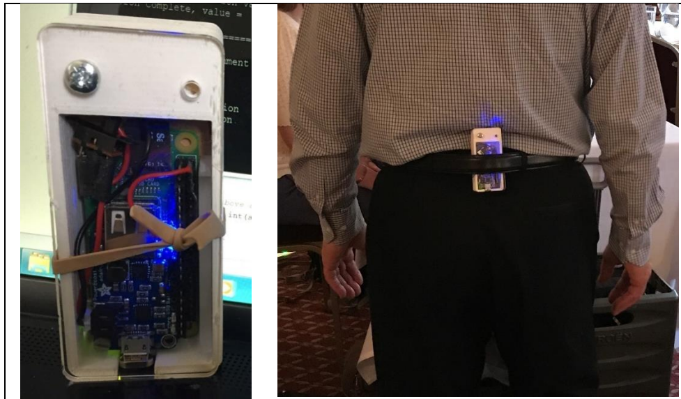
Figure 5.7. Early prototype rider IMU case and dismantled feasibility testing.
