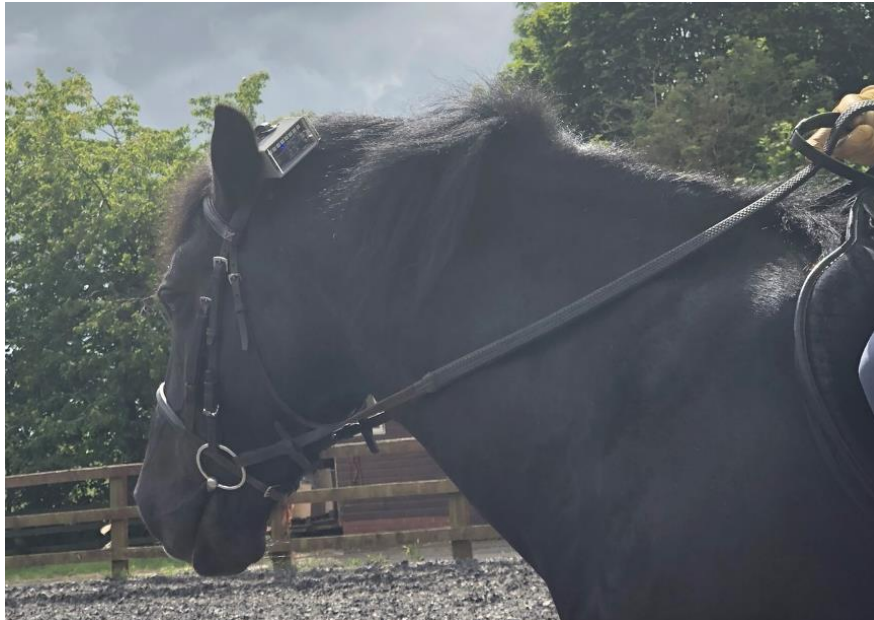
Figure 7.9. LED device obscured by thick mane in windy conditions.
