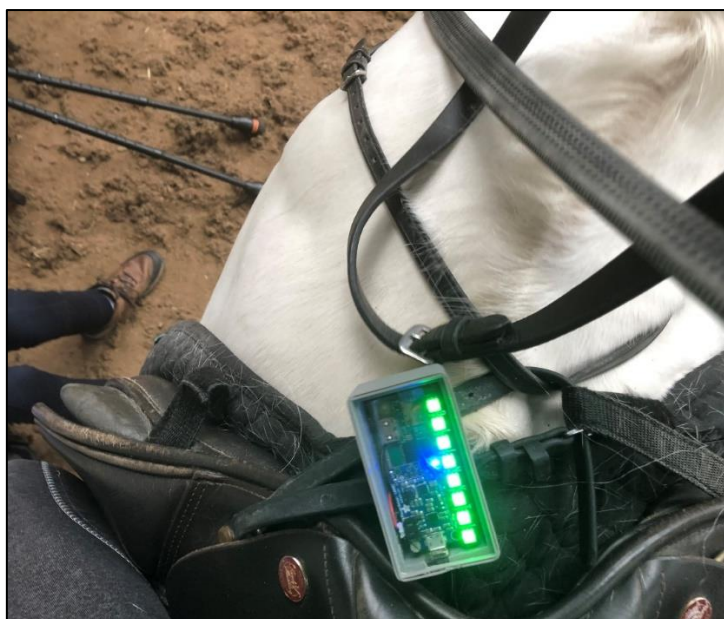
Figure 6.1. Alternative attachment for horse who would not tolerate device on head.
