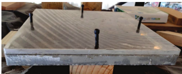
FIGURE 1 | Aluminum manual compression die with tightening screw closed setup.
