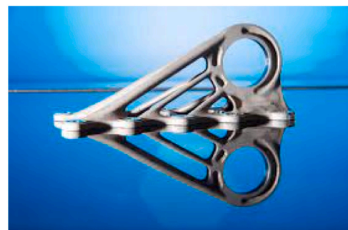
Fig. 12. Topology optimized and additively manufactured Airbus A350 XWB cabin bracket connector by LPBF of Ti6Al4V. Adapted from Ref. [142]. Copyright 2016 airbus.
