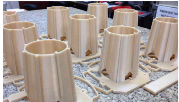
Fig. 9. Antenna arrays for satellites by FDM. Adapted from Ref. [78]. Copyright 2019 Stratays.
