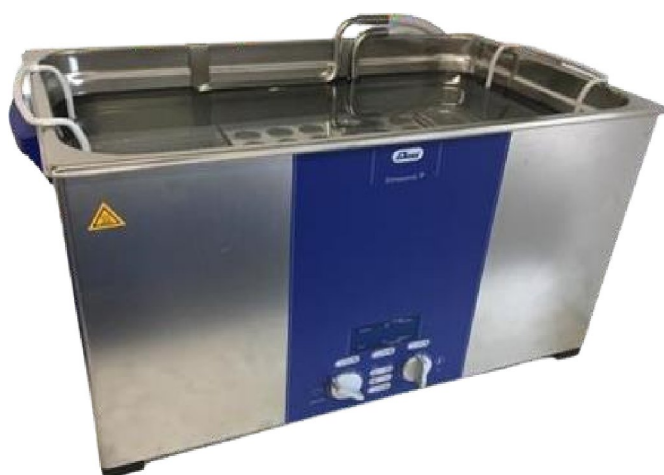
Figure 4. 1: Elmasonic P ultrasonication bath used in this study (University of Sunderland) for the sonication process.
