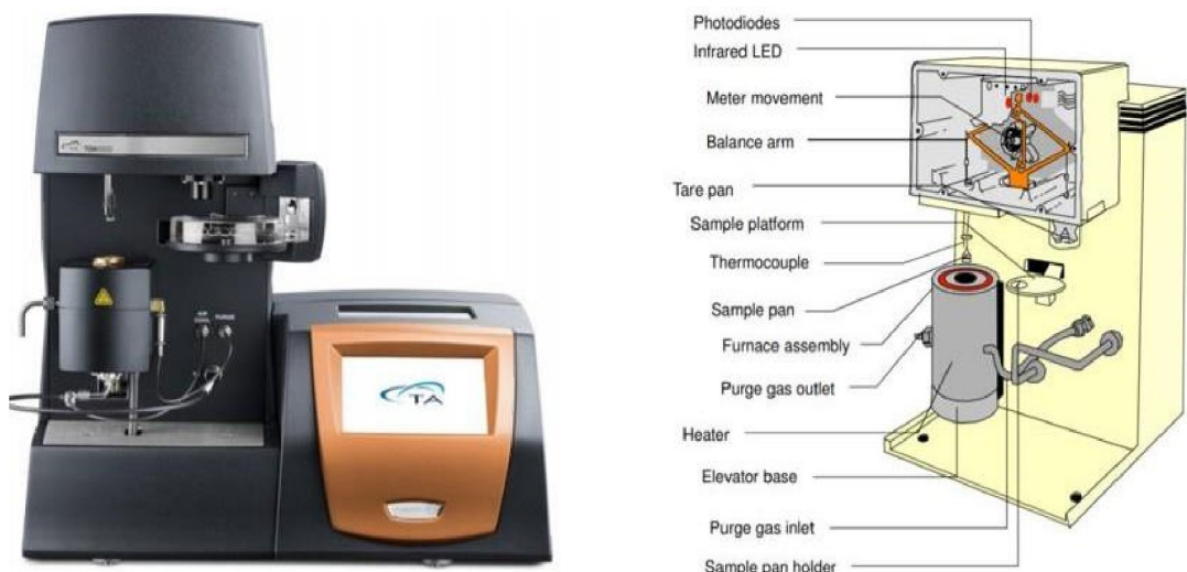
Figure 4. 9: TGA system that was used in this study (University of Sunderland and Schematic (Mohomed, 2016).
