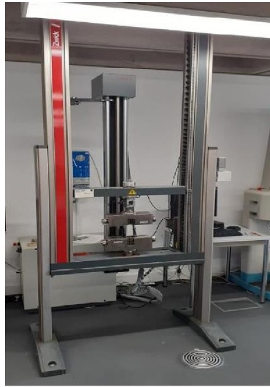
Figure 4. 11: Zwick system that was used in this study (University of Sunderland) for mechanical testing.
