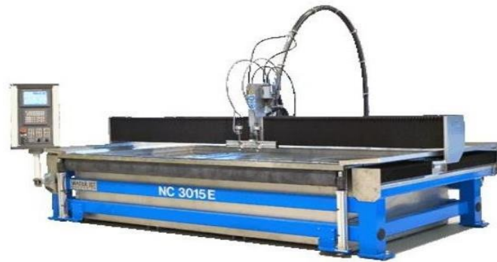
Figure 4. 3: The water Jet Cutting machine used in the present study (National Glass Centre, University of Sunderland).
