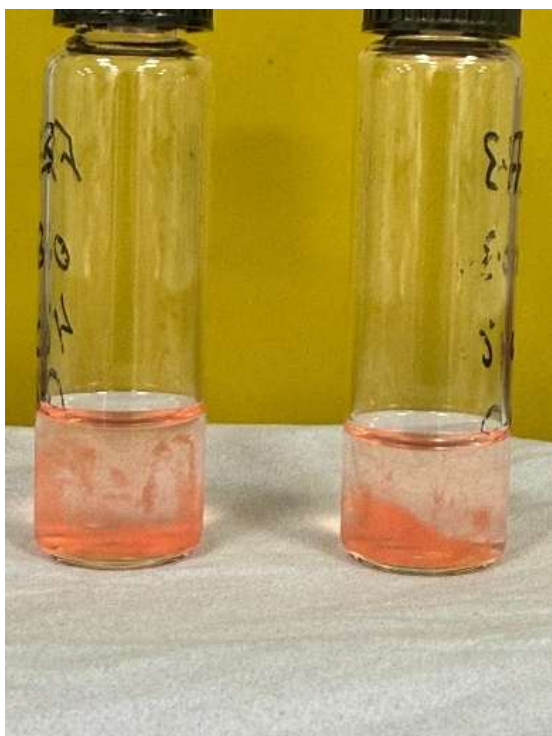
Figure 5.4: Aggregation of niosomes in NaCl solution for formulation loaded at doxorubicin concentration of 0.3 mg/mL (two runs)
