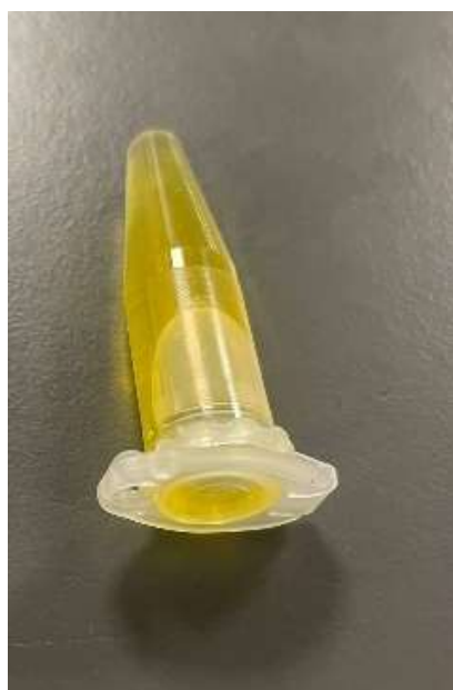
Figure 3.11: Cholesterol, Span 60, Solutol HS15 added to water and sonicated with BCG (0.1mg/mL) after the addition of HCl (0.1 mL of 1 M). The formed suspension changed and stayed yellow.
