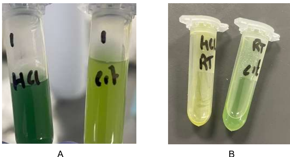
Figure 3.12: In figure 3.12-A, the F6 formulation after 15 minutes of adding HCl (left Eppendorf) and the F8 formulation after 15 minutes of adding citric acid (right Eppendorf). %EE after 15 minutes for F6 is 68.59% and for F8 is 14.86%. In figure 3.12-B, F6 (left Eppendorf) and F8 (right Eppendorf) formulation after 60 minutes of adding HCl (left Eppendorf) and citric acid (right Eppendorf). %EE after 60 minutes drug loading under pH gradient for F6 is 34.61% and for F8 is 29.63% [1] .
