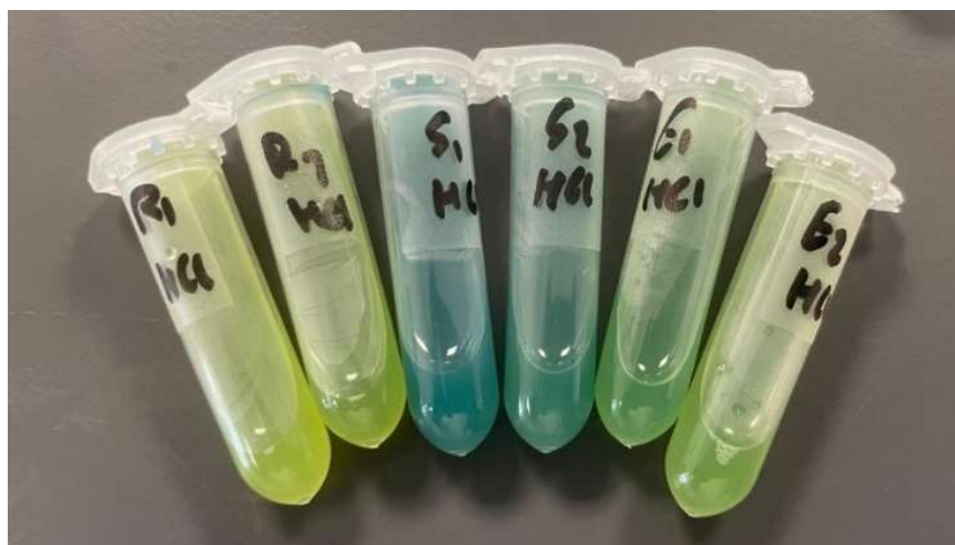
Figure 3.6: The change that occurred in 3 sonicated formulations (from left to right: 2 repeats for F1, two repeats for F3 and two repeats for F2) upon the addition of HCl. HCl was added to these formulations after sonication. The picture was taken 15 minutes after the addition of 0.1 mL of 1 M HCl. %EE reported after sonication after 15 minutes of drug loading is F1= 15.57%, F2= 17.81% and F3= 67.86% [1] .
