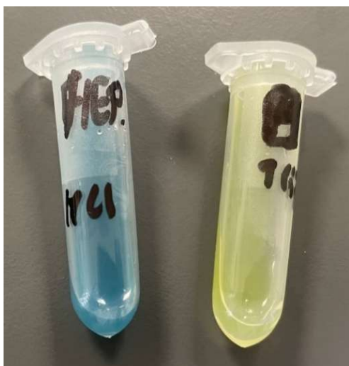
Figure 3.13: Right Eppendorf presents F6 (in trizma buffer) after 1 hour of adding HCl. Left Eppendorf indicates F10 (in HEPES buffer) after 1 hour of adding HCl. The % F6 EE after 1 hour of drug loading was 34.61 %, while that of F10 after 1 hour of drug loading was 72.85 %.
